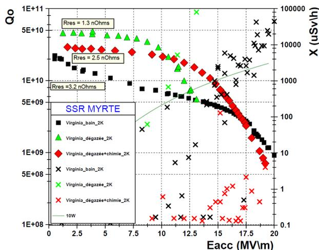
Figure 8:  $Q_0$  factor at 2K versus accelerating gradient of an MYRRHA SSR prototype before hydrogen degassing (black squares), after 600°C degassing during 10h without post BCP etching (green triangles) and with post BCP etching (red diamonds). Field emission is represented by crosses with corresponding colours. Presented at [16].
