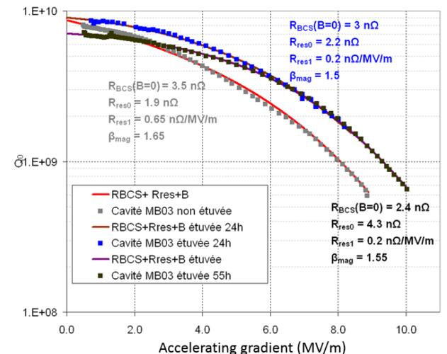
Figure 11:  $Q_0$  at 4.2K versus accelerating gradient of a QWR prototype for Spiral2 project before (grey squares) baking, after 24h (blue squares) and 55h (black squares) at 120°. This cavity has not been hydrogen degassed (figure extracted from [20]).
