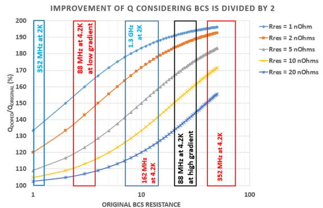
Figure 14:  $Q_0$  gain versus the BCS resistance for different residual resistance. Here the assumption is a reduction of a factor of 2 of the BCS resistance.
