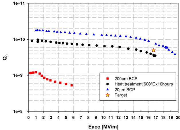
Figure 9:  $Q_0$  at 2K versus accelerating gradient of the low beta elliptical cavity for ESS project before hydrogen degassing (red squares), after degassing (black circles) and after additional BCP etching (blue triangles). Figure extracted from [18].
