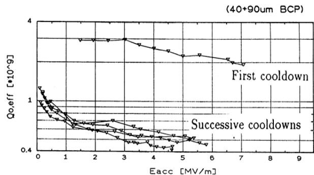
Figure 2: Irreversible degradation caused by hydrogen precipitation of an elliptical cavity after successive cooldown (figure extracted from [2])
