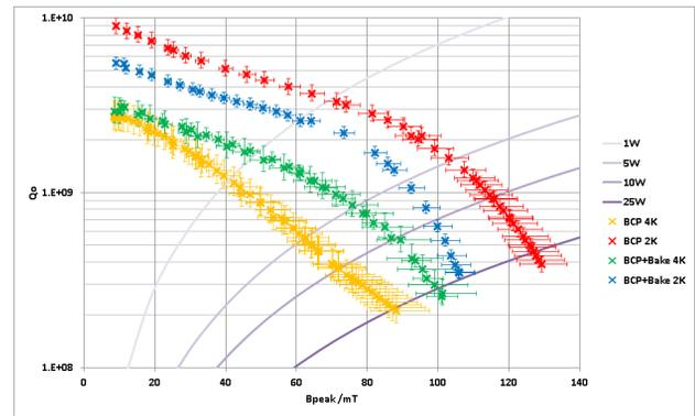
Figure 10:  $Q_0$  versus accelerating gradient of the QWR prototype for RISP project before (yellow squares at 4.2K and red squares at 2K) and after 120°C baking (green squares at 4.2K and blue squares at 2K). This cavity has not been hydrogen degassed. Figure extracted from [19].
