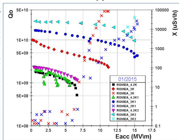
Figure 7:  $Q_0$  factor at 2K versus accelerating gradient of an ESS DSR prototype after a warm BCP etching inducing hydrogen pollution (red diamonds), after a cold BCP etching (blue circles) limiting hydrogen pollution and finally after hydrogen degassing at 600°C during 10h followed by a 30 microns BCP etching (blue triangles). Respectively at 4.2K, black squares, green triangles and purple triangles. Presented at [16].
