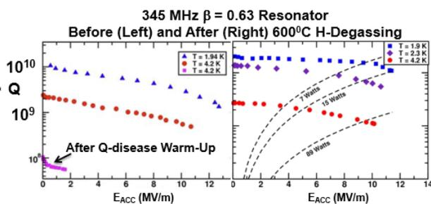
Figure 6:  $Q_0$  versus accelerating gradient before (left) and after (right) hydrogen degassing at 600°C. At 4.2K, surface resistance is dominated by BCS contribution and is decreased of 50%. At 1.9K, residual contribution is divided by a factor of 2 (figure extracted from [13]).
