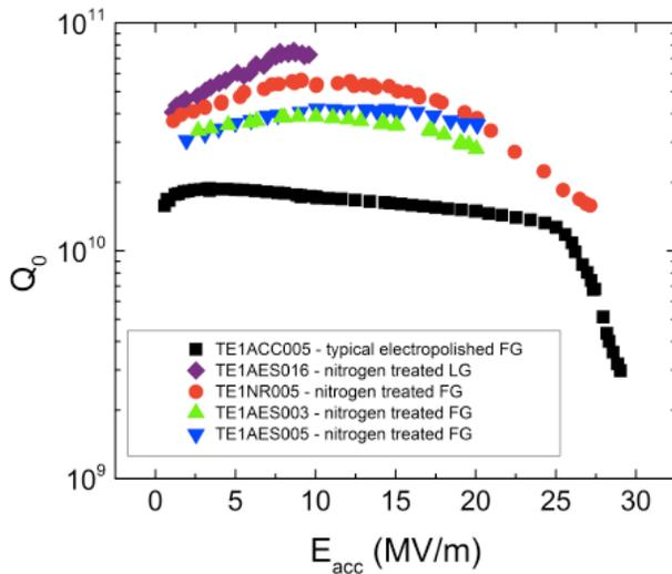
Figure 4: Improvement of the quality factor at 2K thanks to nitrogen doping. In black, the typical Q-curve of a cavity treated with standard recipe (figure extracted from [5]).
