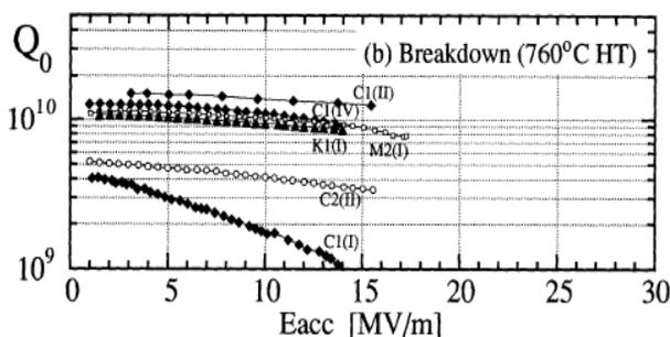
Figure 1: Study of the effect of heat treatments done on elliptical cavities at KEK in 1993. Curve C1(I) and Curve C1(II) represent respectively the quality factor at 2K versus accelerating gradient of a non-degassed and 760°C degassed cavity (figure extracted from [1]).
