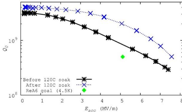
Figure 12:  $Q_0$  versus accelerating gradient of a QWR prototype for ReA3 project before (black cross) and after (blue cross) baking at 120° during 48h. Figure extracted from [22].
