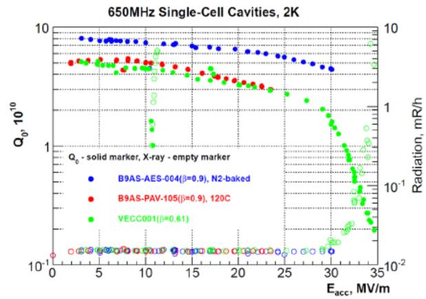
Figure 13:  $Q_0$  versus accelerating gradient of an elliptical cavity at 650 MHz for PIP2 project after hydrogen degassing (green circles), after 120°C baking (red circles) and after nitrogen doping (blue circles). Figure extracted from [23].
