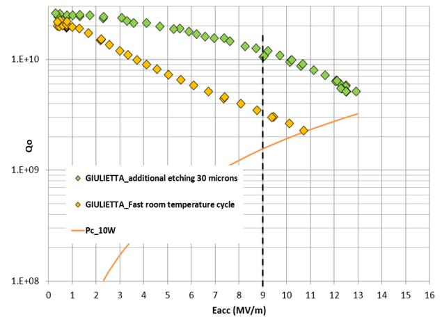
Figure 5: Degradation of the  $Q_0$  visible at 2K after a room Temperature cycle of a double Spoke resonator for ESS.
