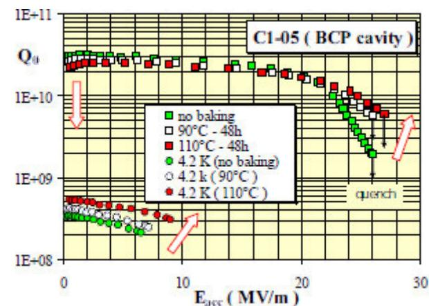
Figure 3: Improvement of the BCS resistance with a 110°C baking during 48h. A  $Q_0$  improvement at 4.2K is the sign of reduction of BCS resistance. A  $Q_0$  degradation at 2K is sign of residual resistance increase (figure extracted from [4]).
