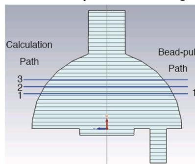
Figure 4: Paths of Bead-pull measurement (right side) and frequency shift calculations (left side).
