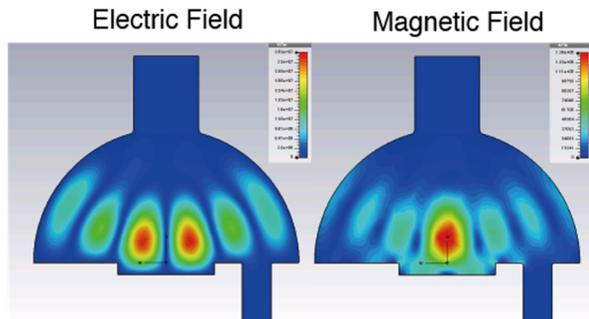
Figure 1: Electric and Magnetic field in mushroom-shaped cavity.
