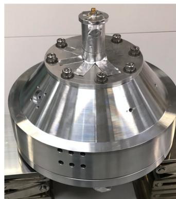
Figure 3: Picture of mushroom-shaped Aluminum cavity.
