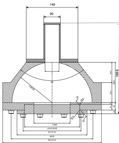
Figure 2: Cross-sectional drawing of mushroom-shaped Aluminum test cavity.
