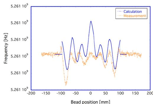
Figure 5: Comparison of bead-pull frequency shift between bead-pull measurement (orange) and CST calculation (blue), at 5.261GHz mode.
