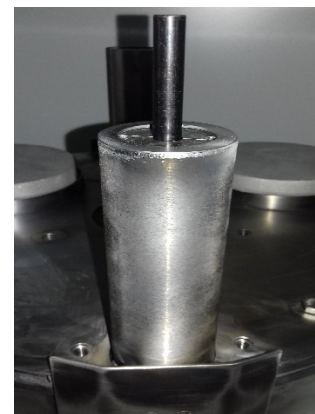
Figure 1: Coated srf-gun dummy sitting in its specially designed coating sample holder system.
