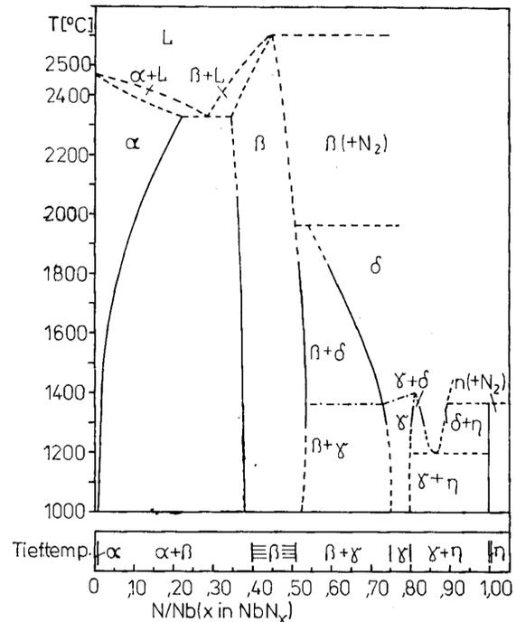
Figure 1: Phase diagram of NbN. The δ-phase of NbN forms at temperatures between 1300°C and 1700°C [3].
