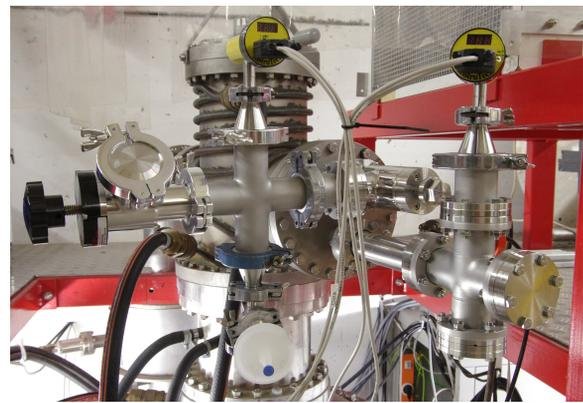
Figure 7: Nitrogen supply system at the top of the furnace. As only a small volume is required, it consists of a KF40 cross in the center with attached periphery: At the top a Pirani vacuum gauge, on the left a vacuum valve for a vacuum pump, at the bottom a nitrogen inlet with particle filter.
