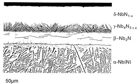
Figure 2: Cross section of the microstructure of NbN. The sc δ-phase forms at the highest nitrogen concentration at the top, followed by the nc β-phase and the sc α-phase at the bottom. During cooldown the δ-phase transforms into the sc γ-phase [4].
