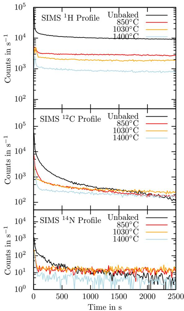
Figure 6: SIMS depth profiles of impurities for different temperatures. Compared to the unprocessed sample (black) the impurities get pushed out. Note that these measurements only allow a qualitative comparison.
