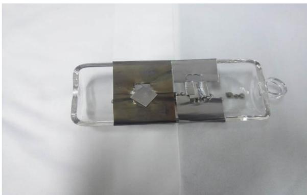
Figure 4: Two niobium samples were placed over the tin source.
