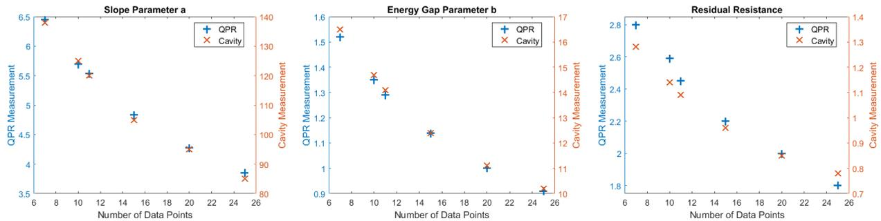
Figure 3: Random error amplification factor  $\alpha$  defined by the ratio of standard deviation of a fit parameter normalized to the true value and random input error (see Eq. (10)).
