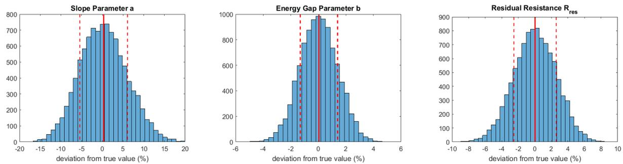
Figure 2: Distribution of fit parameters for Eq. (1) for 10,000 fits with random input error of 1% and 10 data points in the temperature range of 2.0 – 4.5 K. Mean and standard deviation are highlighted by vertical lines.
