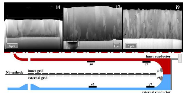
Figure 4: FIB cross-section of samples coated with DC bias diode baseline (single cathode) from [12].
