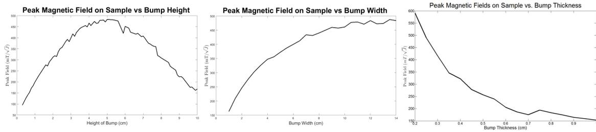
Figure 4: Peak surface magnetic field on sample for 1 J in the cavity. In each plot the unlisted dimensions are Height = 3 cm, Width = 6 cm, and Thickness = 0.3 cm. There is some noise in simulated data due to meshing.
