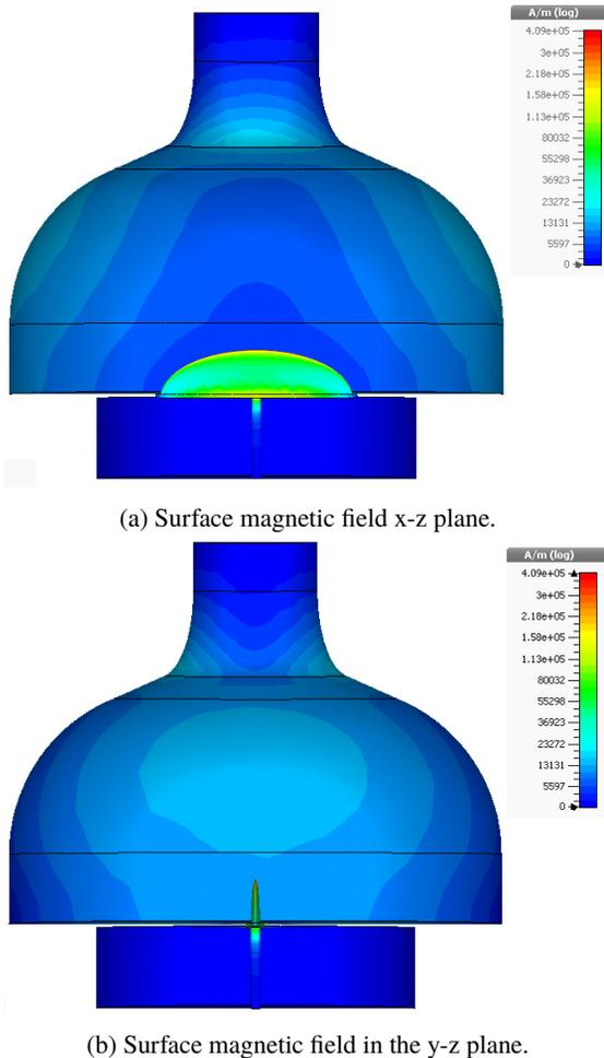
Figure 5: Surface magnetic field in upper and lower cavities.
