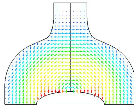
(a) The electric field pattern x-z plane.
