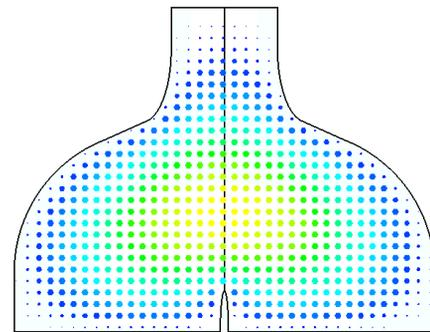
(b) The electric field pattern in the y-z plane.
