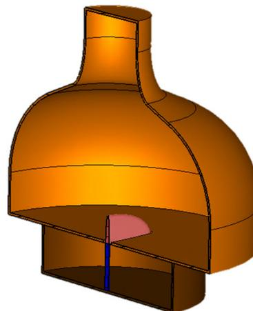
(a) Cross section of whole cavity. Note upper and lower chambers
