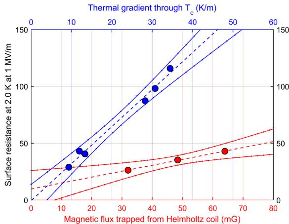
Figure 2: Measurements of the increase in residual resistance as a function of the applied thermal gradient (in blue) and trapped ambient magnetic field (in red) during the cool-down through  $T_c$ .
