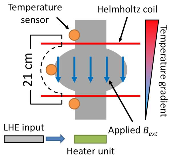
Figure 1: Diagram illustrating the experimental setup of the single-cell cavity. Liquid helium is introduced in a control fashion at the base of the cryostat, which, in the absence of power from the heater unit, allows cooling in an almost-uniform gradient. The Helmholtz coil allows the application of an external magnetic field, whilst the use of the heater develops a temperature gradient across the cavity, measured by the Cernox sensors mounted on the equator and irises.
