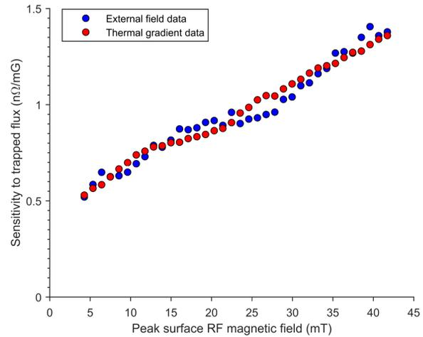
Figure 3: A measurement of the sensitivity to trapped flux, using data from both Helmholtz coil (blue) and thermal gradient (red) cool-downs, as a function of the applied RF magnetic field in the cavity.
