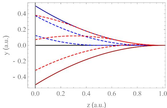
Figure 6: Motion of a flux line under the influence of the RF field in a weak collective flux pinning scenario. During the initial phase, the vortex line is displaced from neutral (blue) until it reaches the peak of its oscillation. As the Lorentz force starts decreasing and the vortex moves in the opposite direction (red), the impact of the weak pinning sites changes the sign of the curvature near the tip of the vortex.
