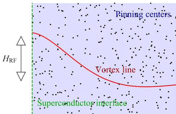
Figure 5: A representation of the weak collective flux pinning model. A vortex line, oscillating under the influence of the RF field, dissipates power into the superconductor due to the force imposed by a high density of weak pinning sites.
