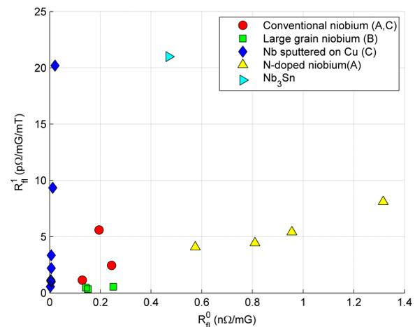
Figure 4: Values from literature for the offset  $R_{fl}^0$  and slope  $R_{fl}^1$  from Equation 1. The legend indicates the source of the data: (A) [7], (B) [8], and (C) [6].
