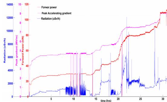
Figure 2: Cavity RF Conditioning history at FREIA.
