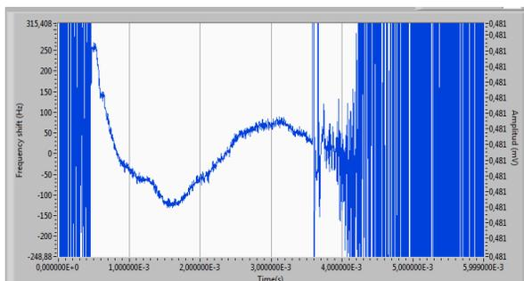
Figure 5: Dynamic Lorentz detuning of ESS spoke cavity during 2.86 ms pulse.
