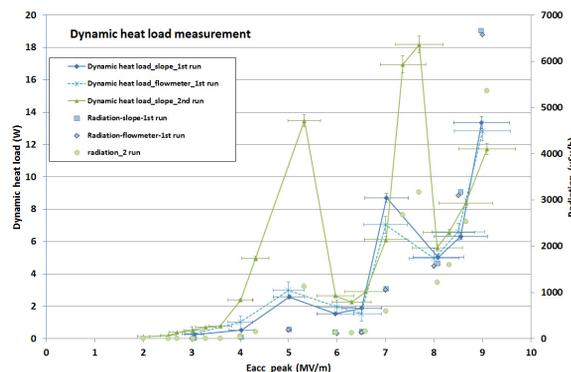
Figure 4: Dynamic loss vs. accelerating gradient.
