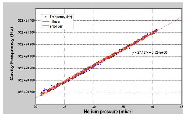
Figure 7: Cavity frequency shift as a function of helium pressure from 20 to 40 mbar.
