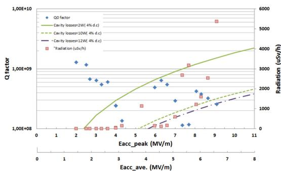
Figure 3: Cavity package performance as a function of accelerating gradient.
