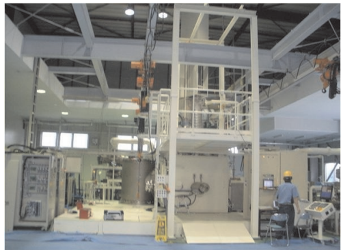
Figure 1: 600 kW electron beam melting furnace [4].
