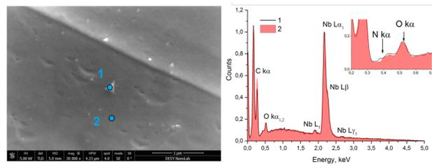
Figure 4: Left: SEM image of the sample which was in the oven with 1DE18. Right: EDX spectrum of two spots on the SEM image. A slight excess of nitrogen at roughly 0.4 keV in such a star-like structure is visible. EDX spectra on other samples were inconclusive, hence no unambiguous identification was possible.
