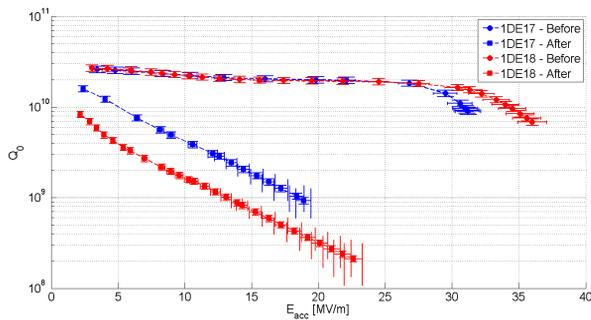
Figure 2: Quality factor vs. the accelerating field of the two single cells, treated in the DESY furnace. Circles are before, squares after treatment, red markers for 1DE18 and blue markers for 1DE17.
