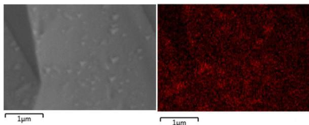
Figure 6: Left: SEM image of the sample which was in the oven with IDE16. Right: EDX map of nearly the same region. One observation, which was not seen in any EDX map before, is an aggregation of carbon at the location of the precipitates.
