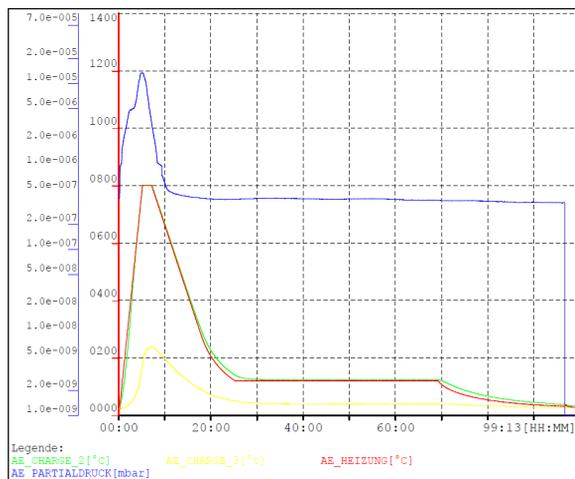
Figure 3: Oven pressure and temperature versus time of the 1DE17 cycle. No nitrogen was injected during the 48h at 120°C bake.
