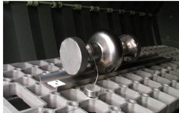
Figure 1: 1DE18 installed in furnace. Two samples are placed in front on a ceramic and the temperature sensor is attached to the cavity.
