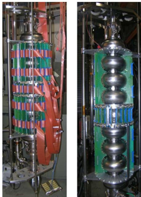
Figure 4: Photograph of the Cornell multi-cell T-Map system.
