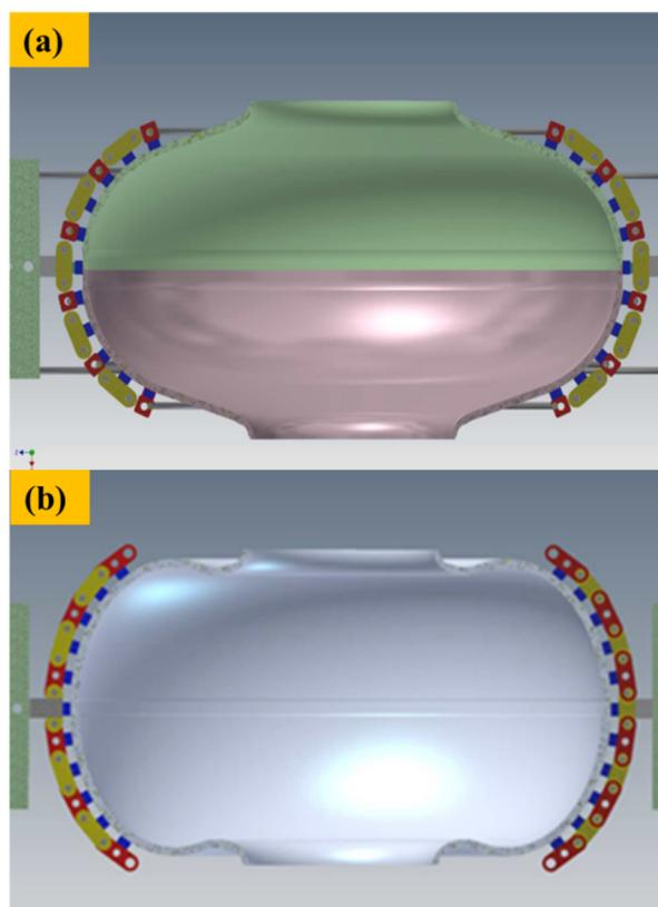
Figure 9: The flexible T-map system fits on (a) a 1.3 GHz ILC-shape SRF cavity; (b) a 1.3 GHz re-entrant shape SRF cavity.
