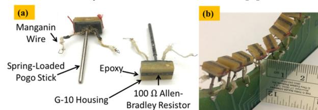
Figure 1: (a) Schematic of a carbon resistor based sensor; (b) Photograph of T-Map sensors with a ruler for size reference.
