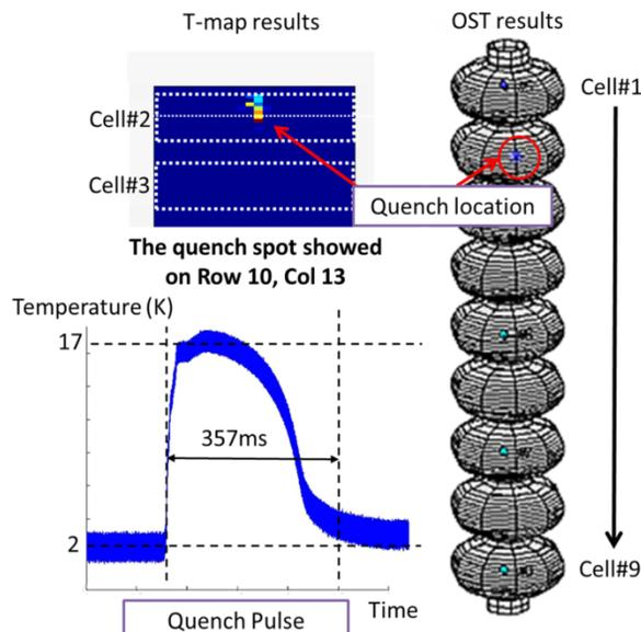
Figure 6: Quench location with TB9AES022 detected by the OST system and the Cornell T-Map with the quench recorded by the T-Map system shown in the inset on the left.
