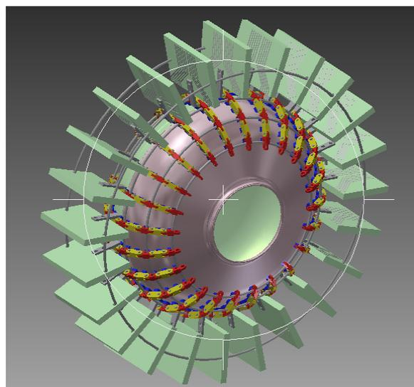
Figure 8: A flexible T-map system with a 1.3 GHz single-cell SRF cavity.
