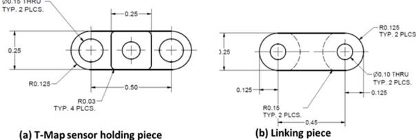
Figure 7: Two different link parts of the expandable chains of the flexible T-map system.
