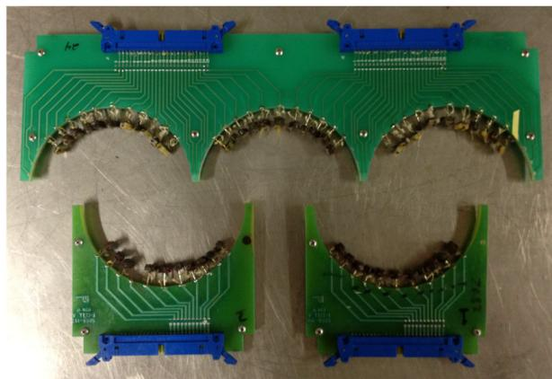
Figure 2: A 3-cell board and a 1-cell board from the Cornell T-Map systems.
