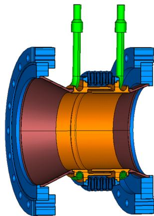
Figure 5: Draft version of the non-collimating shielded bellow with massive copper inner parts (orange), copper-plated tapers (dark red), stainless steel bellow and flange parts (blue) and cooling piping (green).
