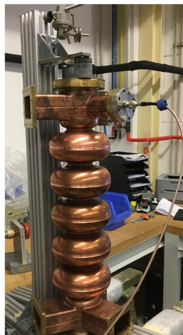
Figure 12: View of the stacked 1.5 GHz 5-cell copper cavity during bead-pull tests at Research Instruments (RI).
