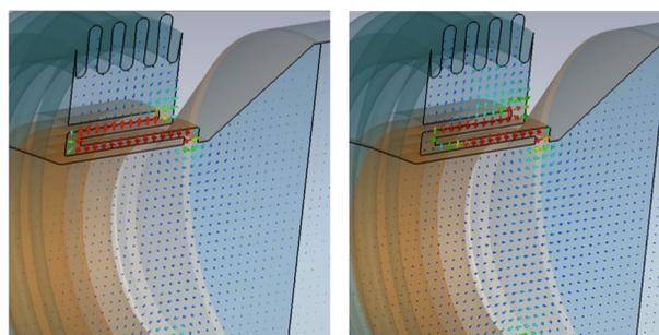
Figure 7: E-field patterns of modes 1 (left) and 2 of the collimating shielded bellow. Mode 2 changes its orientation close to the 180° bend of the labyrinth whereas mode 1 keeps its orientation over the entire length.
