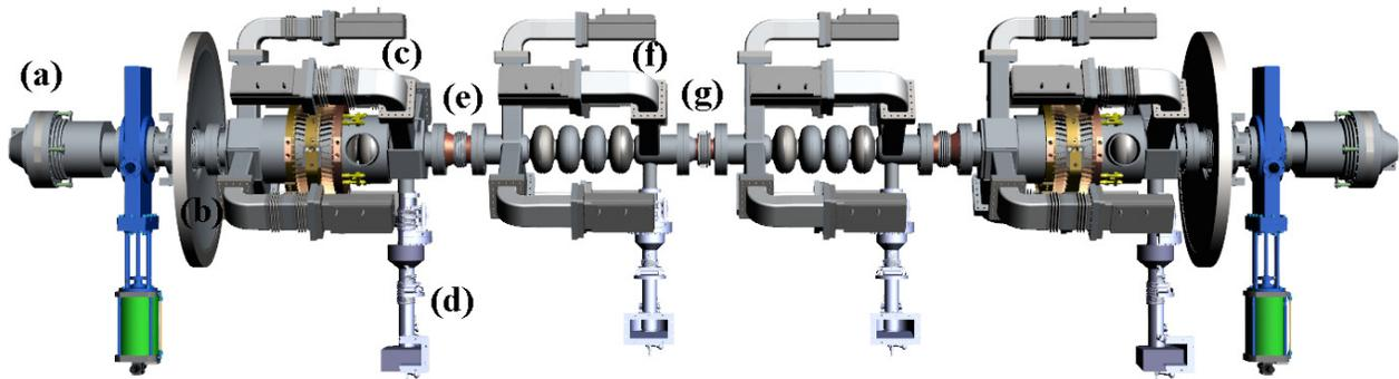
Figure 4: The BESSY VSR cold-string. Components named (left to right): Warm beam-pipe absorber including taper and pumping dome (a). Warm/cold transition bellow (b). 1.5 GHz cavity with He vessel and blade tuner (c). 1.5 GHz, 16 kW high-power coupler (HPC) (d). Non-collimating shielded bellow (e). 1.75 GHz cavity (shown without vessel and tuner) (f). Collimating shielded bellow (g).
