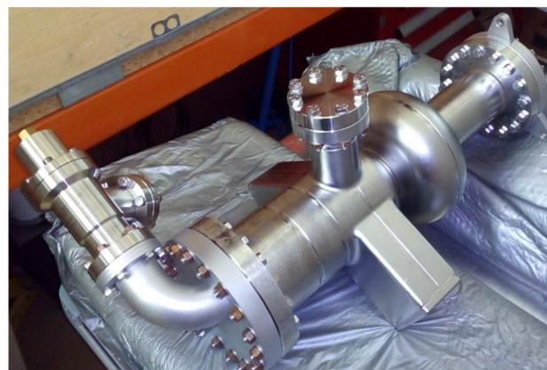
Figure 13: View of the fabricated Nb 1.5 GHz single-cell cavity.
