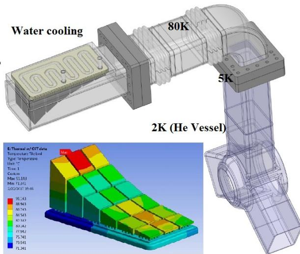
Figure 2: Water-cooled HOM WG loads with calculated temperature rise due to HOM power spectrum (courtesy of F. Fors, Jlab).  $T_{\max} = 91^{\circ}\text{C}$  for 460 W input power.
