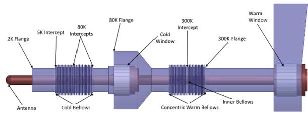
Figure 9: Basic RF design of the 1.5 GHz coupler showing the vacuum and inner conductor. Temperature intercepts and components are clearly labeled.
