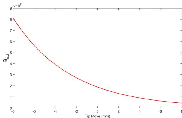
Figure 11: The change in  $Q_{\text{ext}}$  as the coupler penetration depth changes. This corresponds to compression and expansion of the bellows by 10%.
