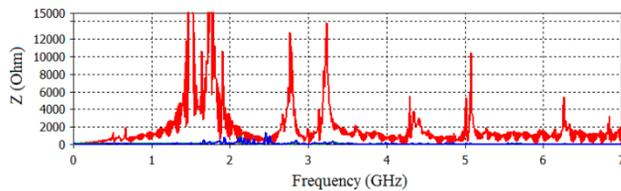
Figure 8: Calculated longitudinal (red) and transverse (blue) impedances for the full BESSY VSR cold-string. Beam harmonics are multiples of 500 MHz and 250 MHz for the “Baseline” and “Extended” baselines [3].
