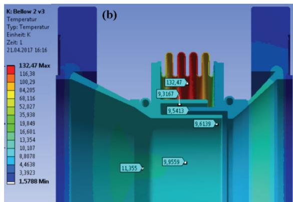
Figure 6: CAD view of the collimating shielded-bellow design (a). Cooling channel are 5...8 K intercepts. Temperature distribution induced by the incident light. The 11.35 K light green area corresponds with the synchrotron light impact point. Heat load on the below section is a result of the fundamental model leaked power (b).
