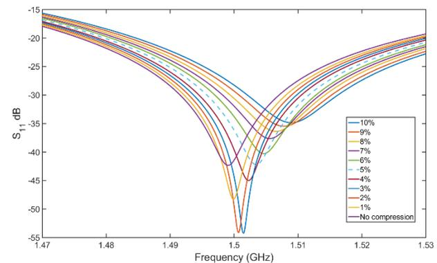
Figure 10: Change in  $S_{11}$  as the bellows are compressed by 10%.
