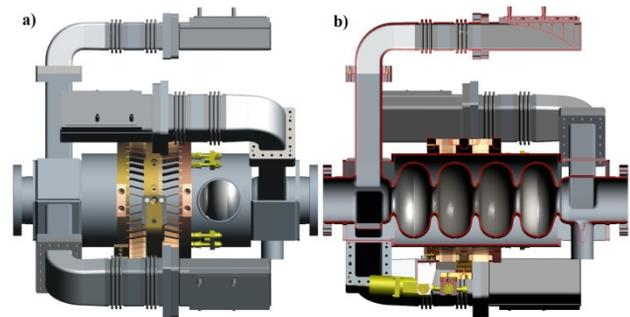
Figure 1: 4-cell 1.5 GHz cavity design equipped with Helvessel and blade tuner (a). Cut plane view showing waveguide (WG) HOM loads design details (b).
