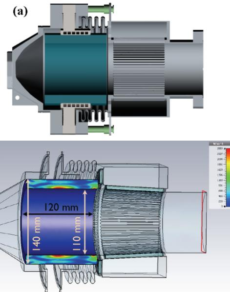
Figure 3: CAD view of the designed warm beam-pipe load (a). Sample EM eigenmode calculation of deposited power densities (b).
