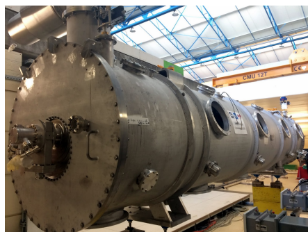
Figure 5: Medium-beta demonstrator cryomodule after completed cavity string insertion and closing of the end flanges in the CEA Saclay test bunker, beginning of July 2017.
