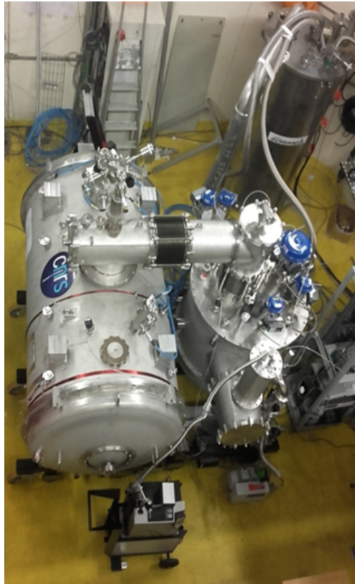
Figure 2: Picture of the spoke prototype cryomodule with the prototype valve box in the test pit at IPN-Orsay.
