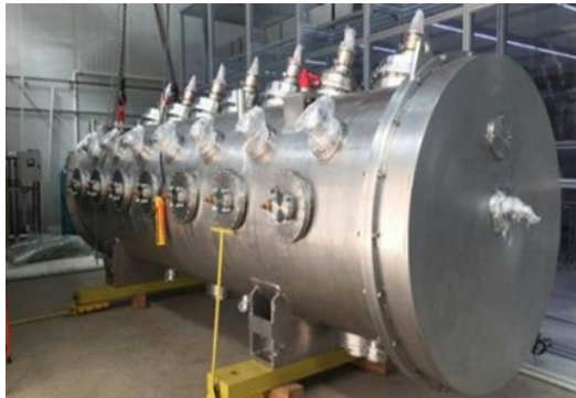
Figure 4: The first cryomodule of Injector-I.
