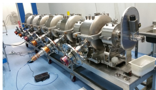
Figure 9: The cavity string of CM4
