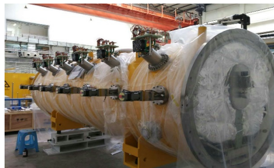
Figure 10: The CM4 cryomodule of 25MeV linac with all the assemblies.
