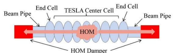
Figure 3: Cavity design scheme of main linac cavity.
