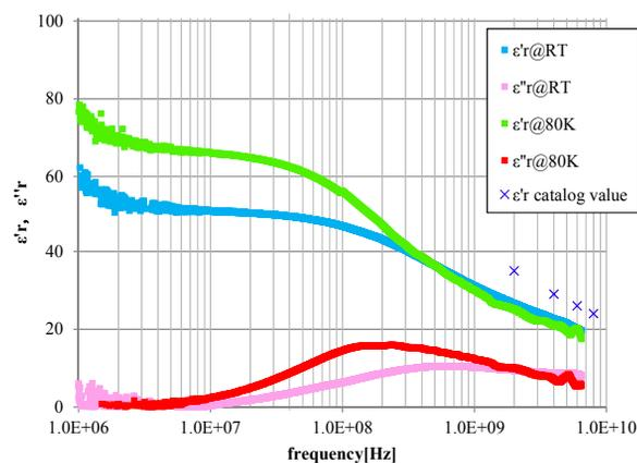
Figure 6: Measured permittivities of AlN at room temperature and 80 K.
