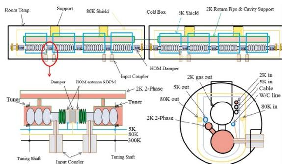
Figure 5: Conceptual design of EUV main linac cryomodule.
