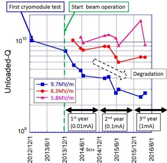
Figure 2: Cavity performance of cERL main linac under cERL beam operation for 3 years.
