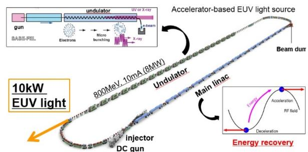
Figure 1: Conceptual layout of accelerator-based EUV light source of more than 10 kW.
