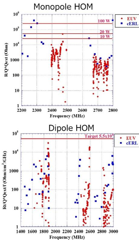
Figure 4: The calculation results of HOM impedances of both monopole modes (top) and dipole modes (bottom).
