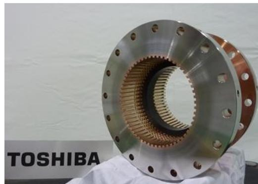
Figure 7: The prototype of HOM absorber.
