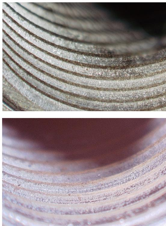
Figure 7: Threads on the TECASINT insert inside the traveling nut (X35 magnification). Top image is an unused nut, and bottom image is nut used for ALT.
