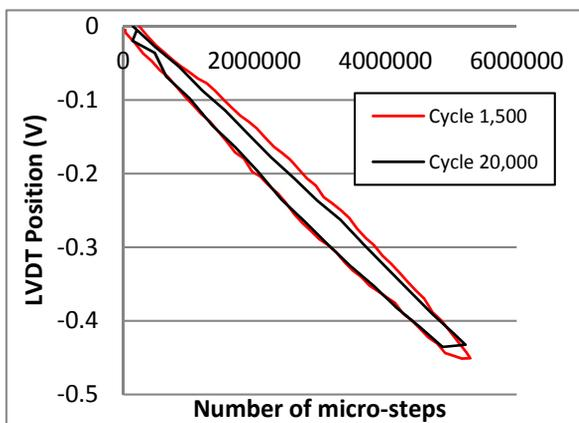
Figure 10: Profile of cycle near the start of and at the end of the experiment.
