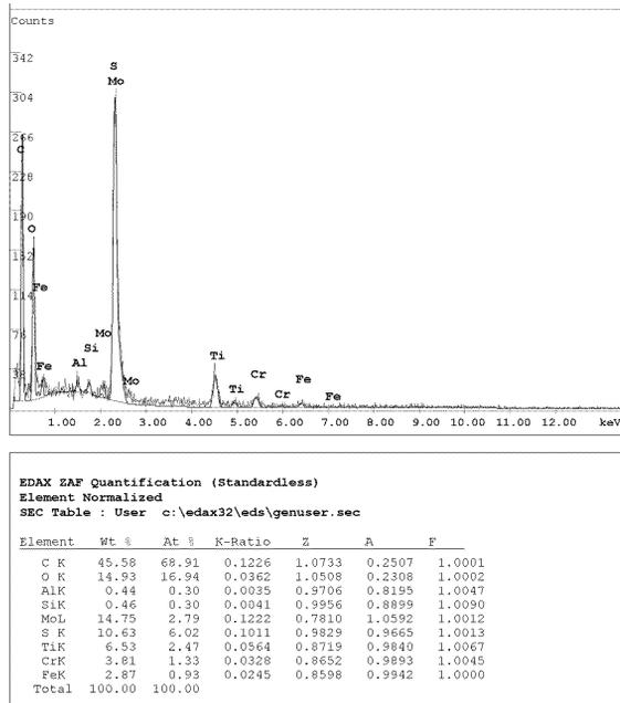
Figure 9: EDS analysis of material found on the spindle.
