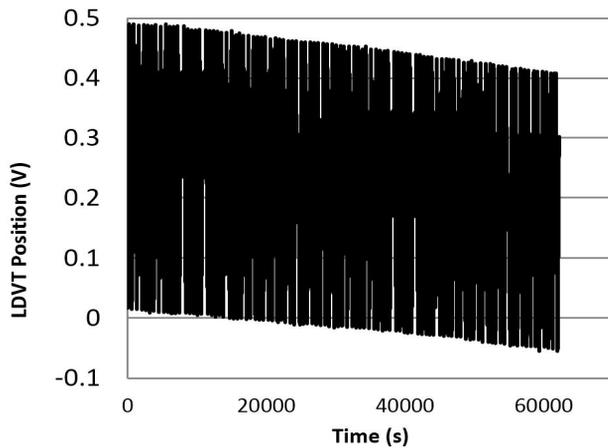
Figure 3: LVDT readings showing drift in tuner testing.
