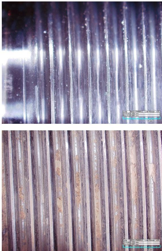
Figure 6: Unused section of the spindle (top) compared with used section of spindle (bottom) under X35 magnification.
