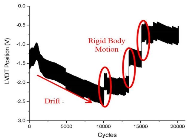
Figure 5: Rigid body motion in LVDT.
