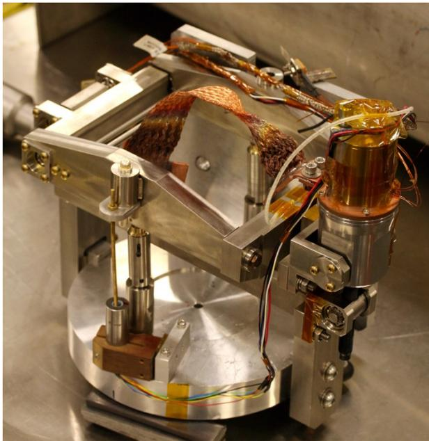
Figure 2: Tuner assembly attached to Aluminium base plate and spring stack for testing.
