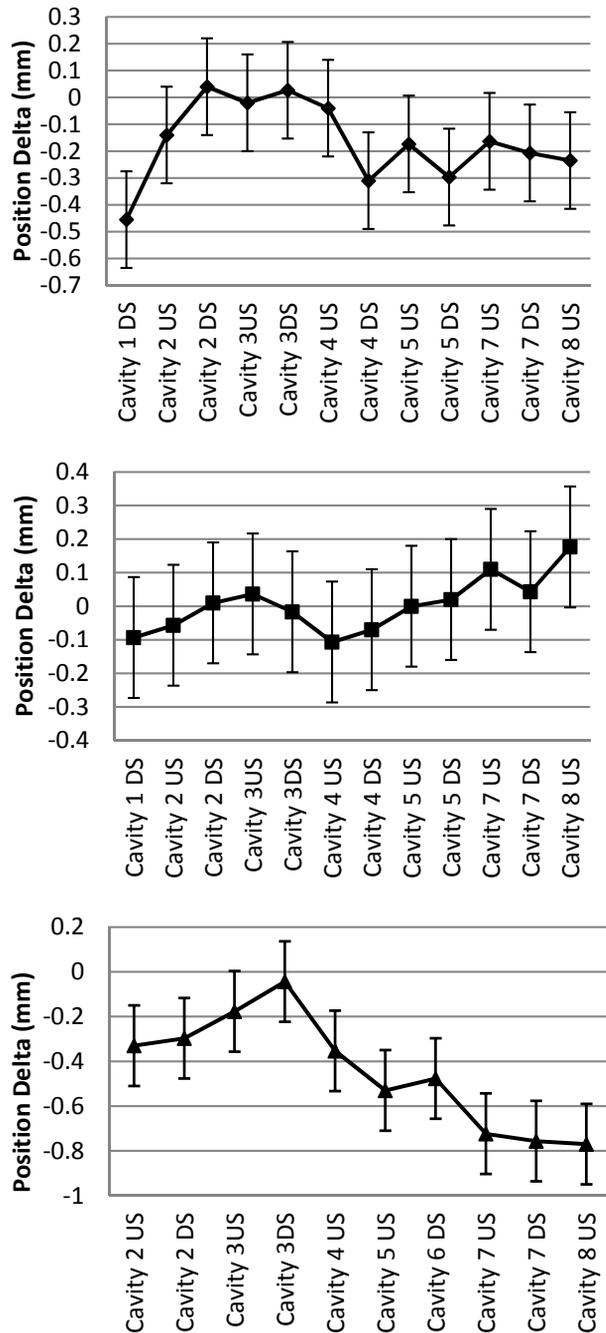
Figure 2: Changes in cavity flange position in the horizontal (top), vertical (middle) and longitudinal (bottom) axes.
