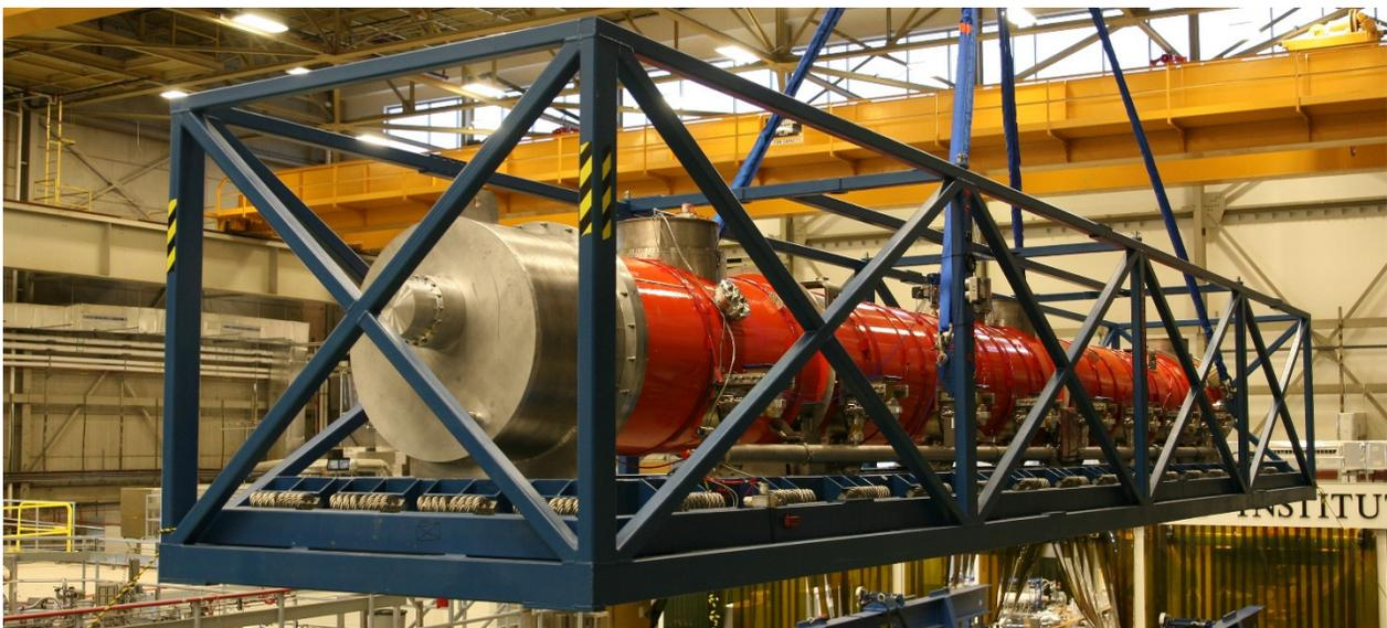
Figure 1: The LCLS-II CM installed in the shipping frame.
