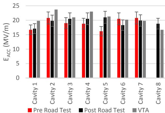
Figure 3: Comparison of cavity gradients before and after road test.
