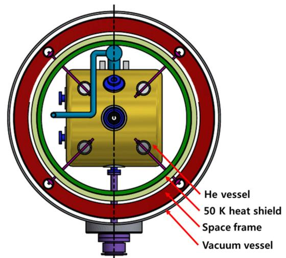
Figure 3: Cross sectional view of the cryomodule.
