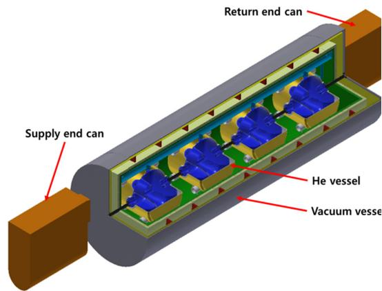
Figure 4: KOMAC HWR cryomodule.
