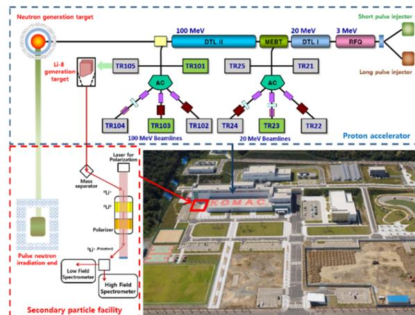
Figure 1: Layout of Secondary Particle Facility.
