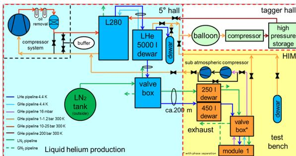
Figure 9: Concept of the cryogenic piping of the test bench at HIM.
