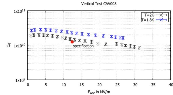
Figure 5: Results of the vertical cryo test of “Cavity 008”. Field emission was seen around 26 MV/m.  $Q_0 = 1.3 \cdot 10^{10}$  at 12.5 MeV and 2 K was reached.
