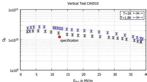
Figure 4: Results of the vertical cryo test of "Cavity 010".  $Q_0 = 1.6 \cdot 10^{10}$  at 12.5 MeV and 2 K was reached.
