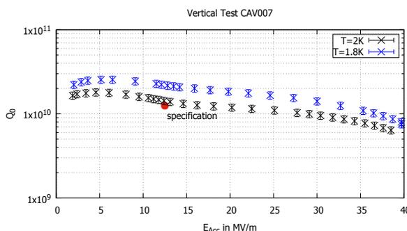
Figure 3: Results of the vertical cryo test of "Cavity 007".  $Q_0 = 1.4 \cdot 10^{10}$  at 12.5 MeV and 2 K was reached.
