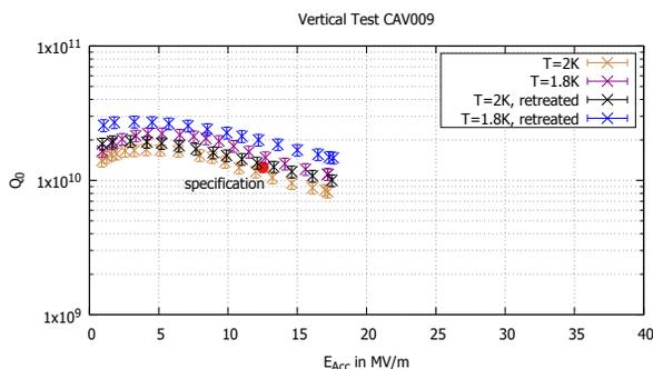
Figure 6: Results of the vertical cryo test of “Cavity 009”. Break down at 16.7 MV/m without Field emission.
