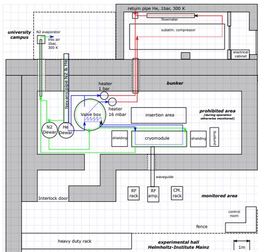
Figure 8: General layout of the SRF test bench at the Helmholtz-Institute Mainz.
