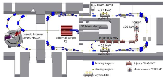
Figure 1: Current design of the MESA lattice. The accelerator is centred around the external beam (EB) mode beam dump. The fixed target experiment P2 is located in the accelerator hall, while the pseudo-internal target MAGIX is located in a separated hall.
