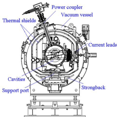
Figure 2: Transverse section of the cryomodule.
