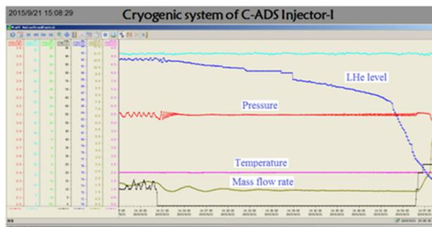
Figure 6: 2 K heat load measurement.
