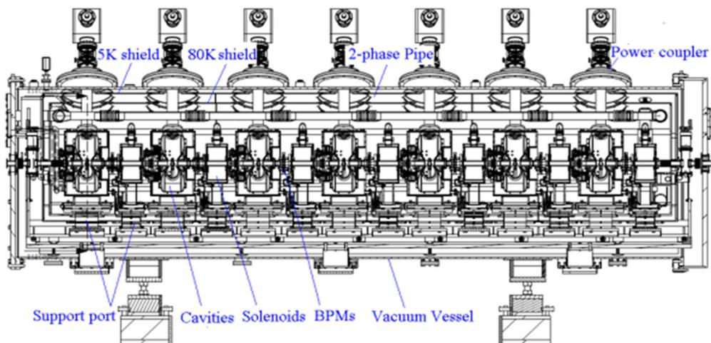
Figure 3: Longitudinal section of the cryomodule.
