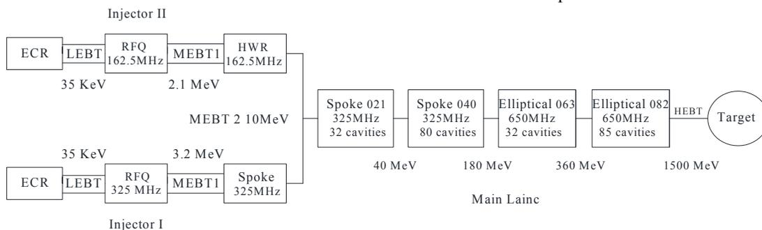
Figure 1: Schematic layout of the C-ADS driver linac.
