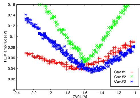
Figure 8: HOM signal v.s. vertical offset.
