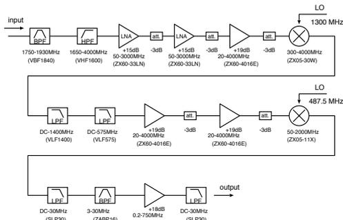
Figure 3: Scheme of the detection electronics.
