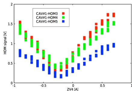
Figure 6: Comparison of HOM ports (vertical scan).
