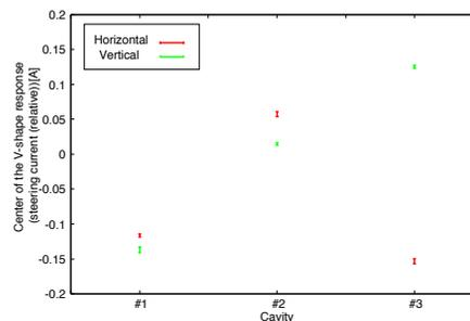
Figure 9: Condition (relative current of the steering magnets) to minimize HOM excitation for each cavity.
