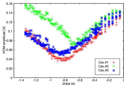
Figure 7: HOM signal v.s. horizontal offset.
