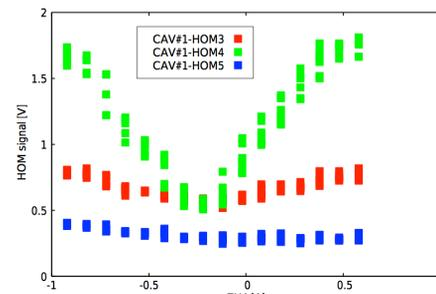
Figure 5: Comparison of HOM ports (horizontal scan).
