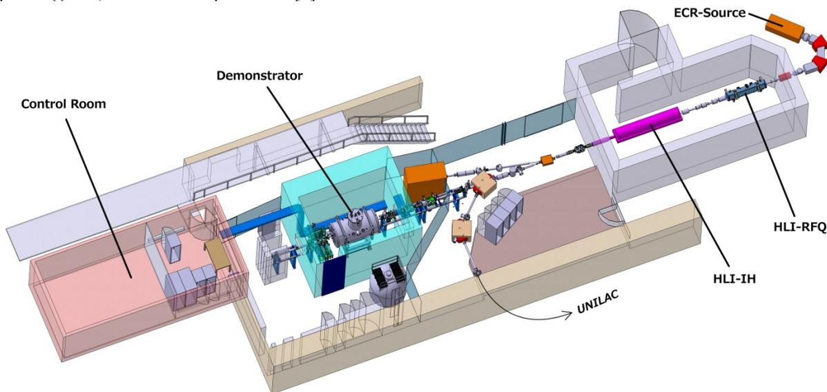
Figure 4: 3D layout of the GSI High Charge State Injector (HLI) with the new cw-LINAC Demonstrator environment
