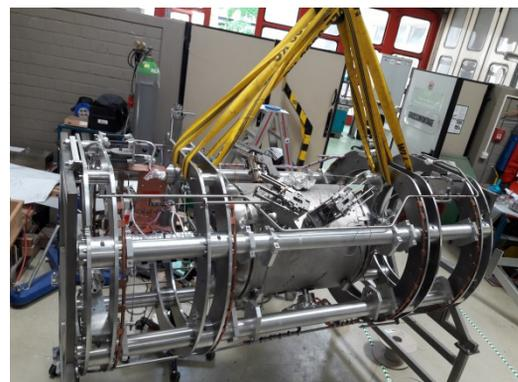
Figure 1: The cw demonstrator comprising a CH-cavity embedded by two solenoids on a support frame, which hang into the cryostat.
