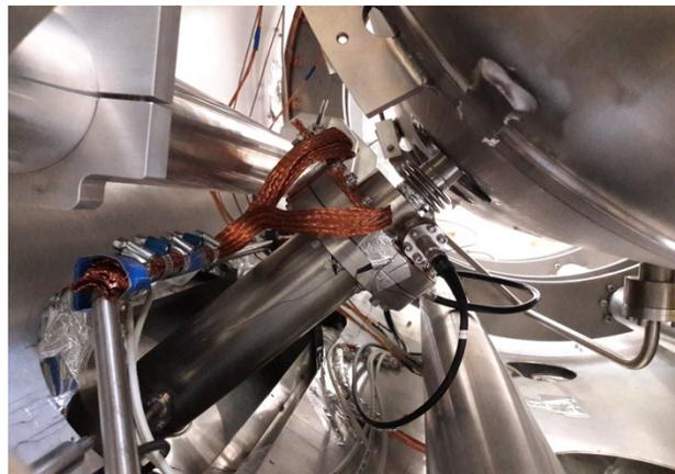
Figure 3: 5 kW power coupler screwed on cavity and cryostat.
