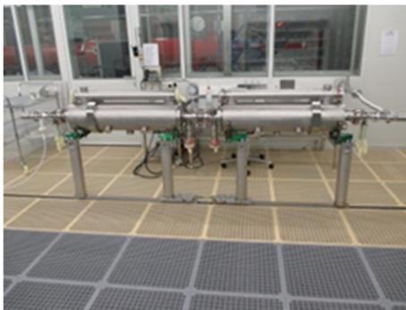
Figure 8: Complete HZDR-String at the pump station in the cleanroom before roll out.
