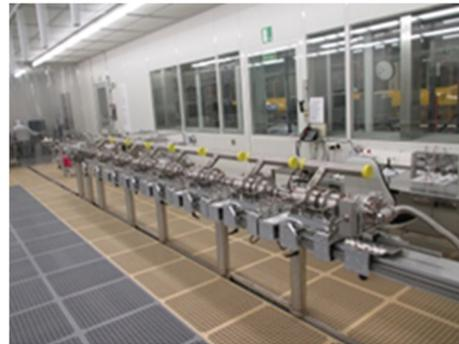
Figure 9: String at the pump station before installation of the last four power couplers.
