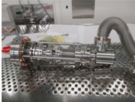
Figure 7: Complete bellow unit for the HZDR-String.
