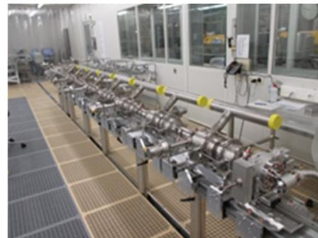
Figure 10: Complete string at the pump station after installed all couplers.
