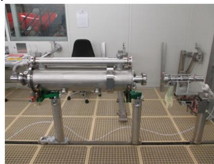
Figure 6: Assembly tool with a bellow unit installed on the extra post.
