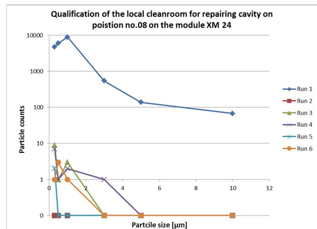
Figure 3: Example of the particle qualification of the local cleanroom for XM24.
