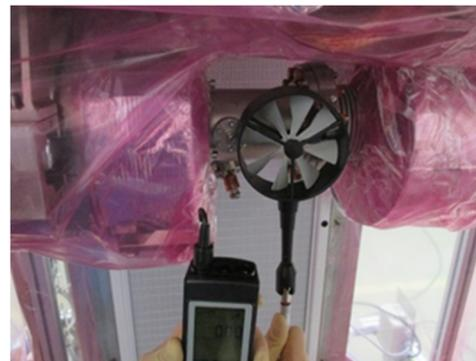
Figure 2: The control of the air flow speed.
