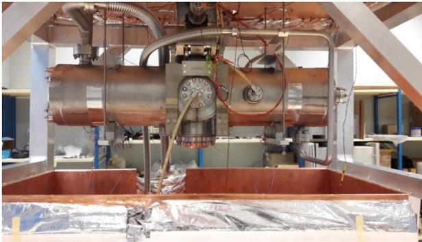
Figure 6: Cavity installed on the top lid cryostat.
