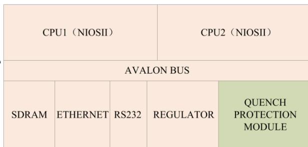
Figure 2: The structure of the digital controller.
