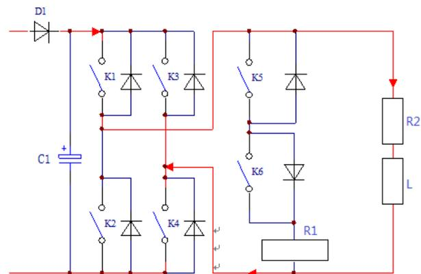
Figure 1: A schematic diagram of main circuit structure.
