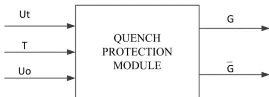
Figure 3: The interface of quench protection module.
