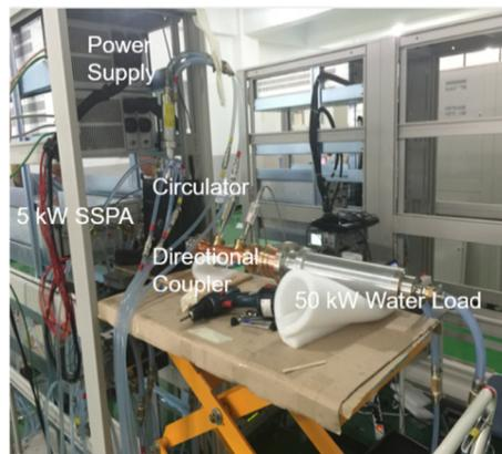
Figure 3: 5 kW Full power test bench.
