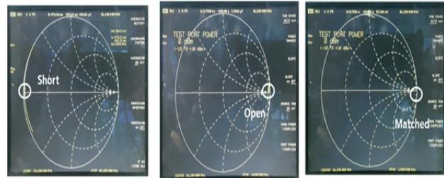
Figure 6: Variable impedance generated by adjusting the movable short device.
