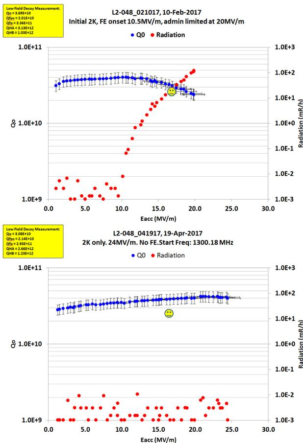
Figure 3: Vertical testing results of a production LCLS-II cavity, as-received (upper plot) and after HPR re-work (lower plot),  $Q_0$ - $E_{acc}$  curve in blue and radiation measurements in red.
