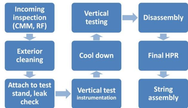
Figure 1: Process flow for LCLS-II cavities after arriving at JLAB from the vendors.
