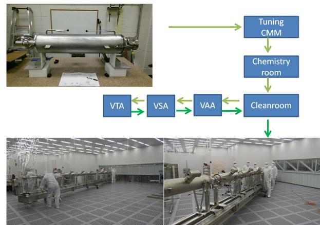
Figure 2: The path of LCLS-II cavities through JLAB work centers, from receiving inspection to an LCLS-II string.
