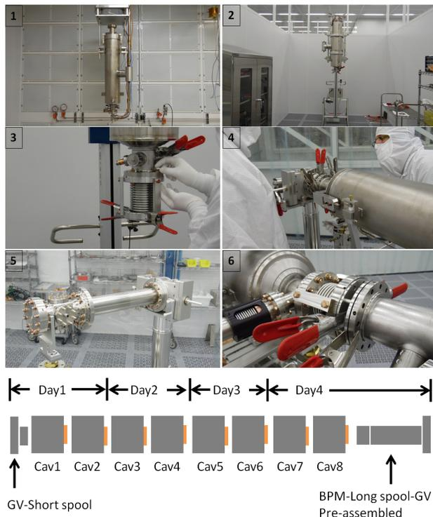
Figure 4: LCLS-II string assembly activities and work flow (lower cartoon). Upper images: 1) A cavity on a test stand at VAA. 2) A cavity received HPR and drying in the assembly cubicle. 3) Vertical assembly of a bellows to a cavity. 4) Horizontal assembly of a cavity beamline flange to the short spool. 5) BMP subassembly. 6) Horizontally connecting of two cavity-bellow subassemblies.
