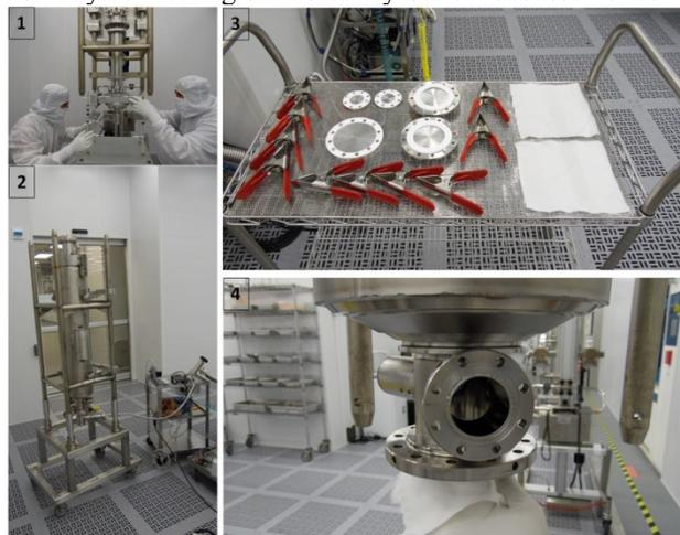
Figure 5: Efforts during LCLS-II string assembly to reduce the chance of particulate contamination: 1) Vertical assembly of a BPM subassembly. 2) Slow venting system, backfill of the cavity to atmosphere pressure with filtered nitrogen. 3) Dedicated covers and clamps used during string assembly. 4) Cleaning the sealing surface after removing the bottom flange, getting ready for the final HPR.
