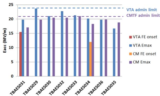
Figure 7: Performance comparison of prototype cavities during VTA final test and prototype CM test.
