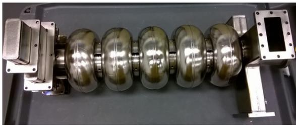
Figure 2: Picture of the fully welded 5C75-003 cavity.
