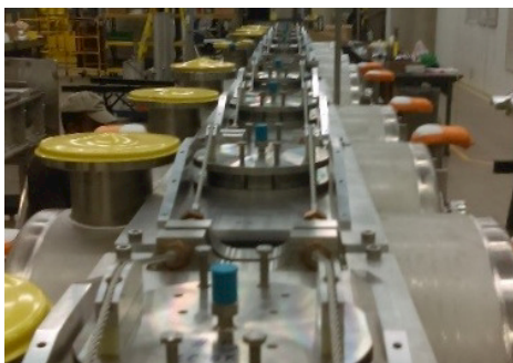
Figure 9: Pneumatic frequency tuner. Helium gas pressurizes the piston actuator, compressing the cavity in the beam line direction by the tuning arms.
