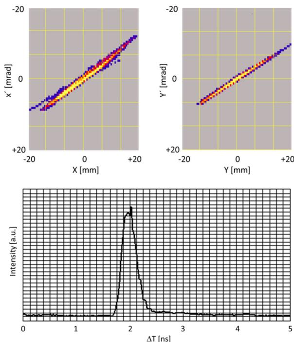
Figure 5: Measured horizontal (top left) and vertical (top right) beam emittance and bunch structure (bottom) for accelerated heavy ion beam behind demonstrator set up.
