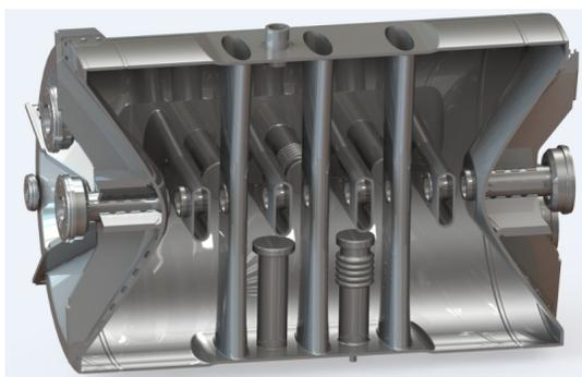
Figure 6: Sectional drawing of the short cavities for CM1 [26].
