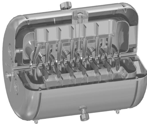
Figure 3: Sectional drawing of the 15-gap demonstrator CH-cavity [19].
