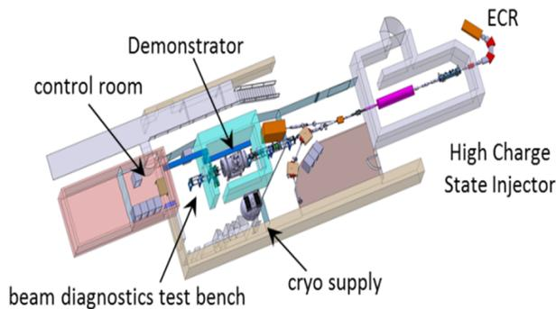
Figure 2: CH-multi cavity test environment@GSI.
