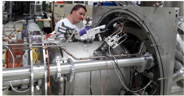
Figure 4: Installation of demonstrator cryo module comprising CH cavity embedded by two sc solenoids on a support frame.
