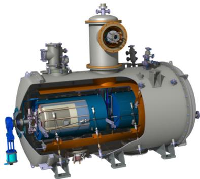
Figure 4: Cut-view of the model of a spokes cryomodule equipped with 2 double-spokes cavities (courtesy IPNO).
