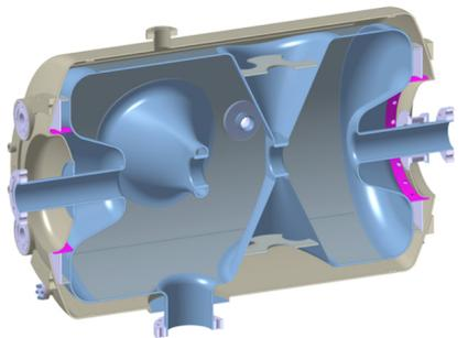
Figure 1: ESS double-spoke cavity cross-section and its helium tank (courtesy: IPNO).
