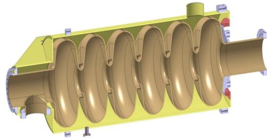
Figure 2: ESS medium- $\beta$  elliptical cavity cross-section and its helium tank (courtesy: CEA).
