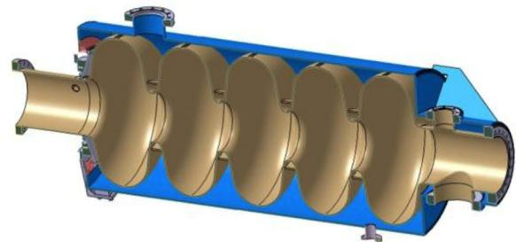
Figure 3: ESS high- $\beta$  elliptical cavity cross-section and its helium tank (courtesy: CEA).
