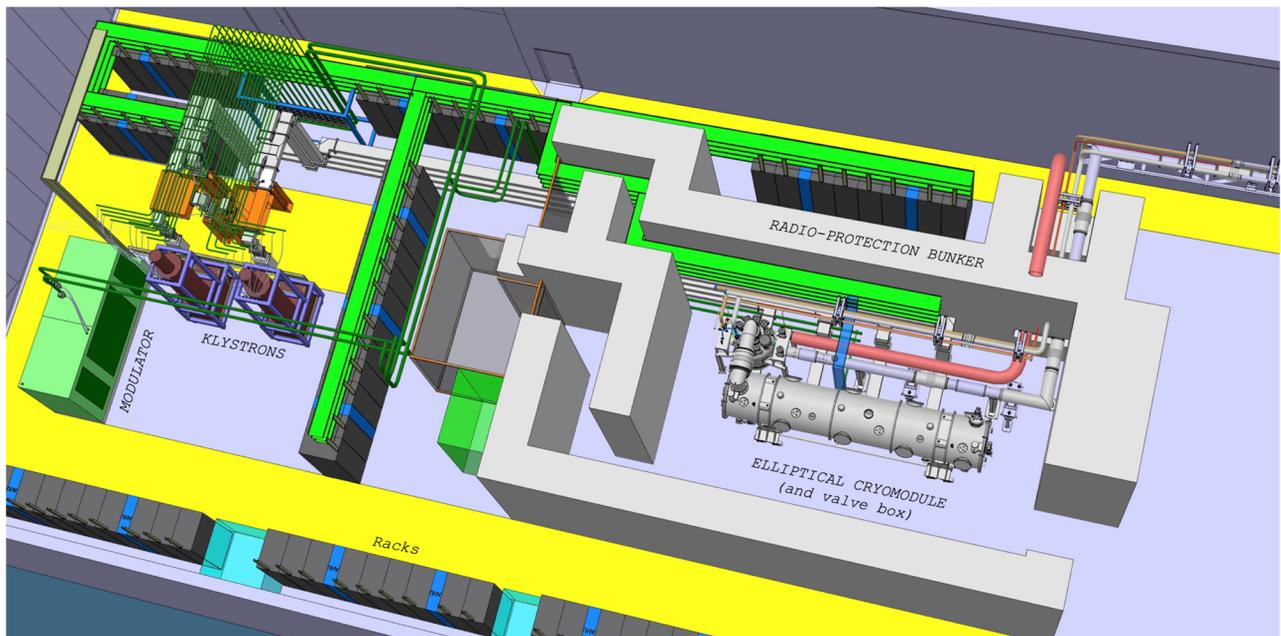
Figure 6: Layout of the ESS Lund Test Stand 2 (TS2). The RF sources shown on left side and bunker with cryomodule under test on the right side.
