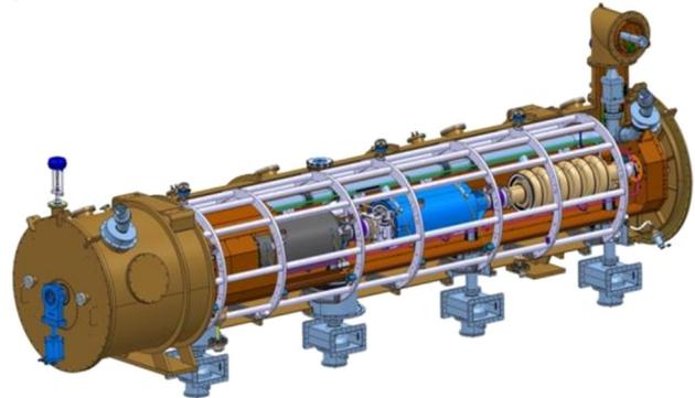
Figure 5: Cut view of the model of an elliptical cryomodule containing 4 medium- $\beta$  cavities (courtesy CEA).
