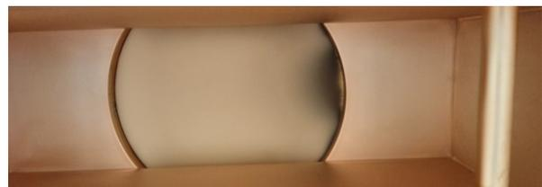
Figure 6: Cavity D damaged RF window.
