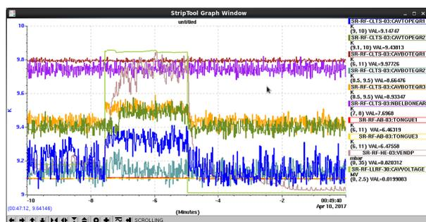
(a) Heating on cavity 3 equator
