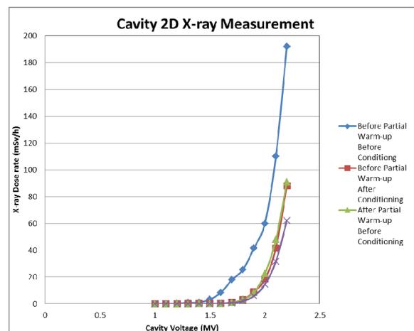
Figure 4: Effect of partial warm-up and conditioning.
