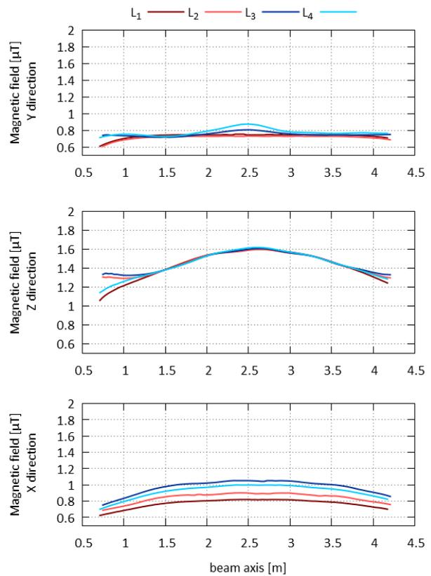
Figure 8 : Magnetic field on HPR port lines for the different external field direction.
