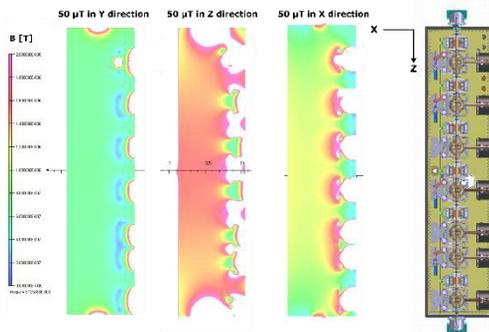
Figure 7: Magnetic field on the plane (X, 0, Z) with an external field of 50  $\mu\text{T}$  on the Y, Z and X direction.
