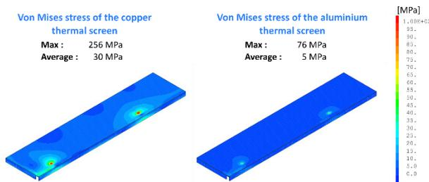
Figure 3 : Von Mises stress of a quarter of the shield top part depending on the material.
