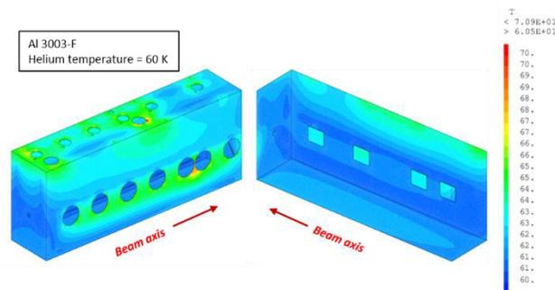
Figure 5 : Temperature of the thermal shield made of Al 3003-F (steady state).
