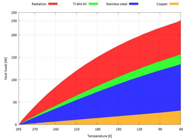
Figure 4 : Heat loads contributions depending on temperature.
