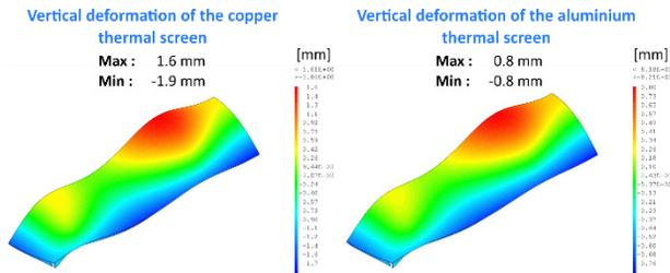
Figure 2 : Vertical deformations of a quarter of the shield top part depending on the material.
