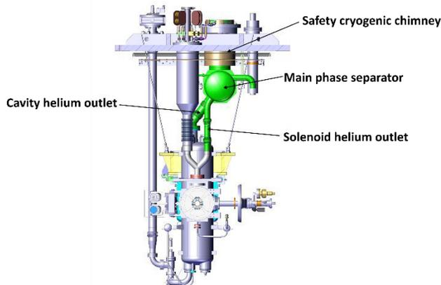
Figure 9: Solenoid and cavity helium outlet.
