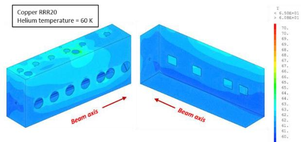
Figure 6 : Temperature of the thermal shield made of copper (steady state).
