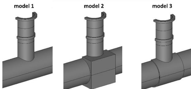
Figure 10: Models used for the simulations of the main phase separator.
