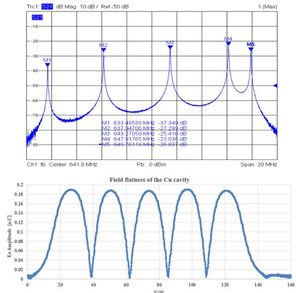
Figure 5: Cu cavity's fundamental spectrum (Top) and the field flatness after it's tuned in RI (Bottom).
