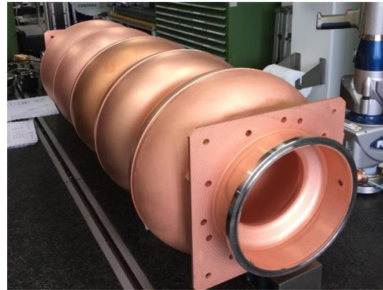
Figure 4: The copper cavity model with detachable end-group.
