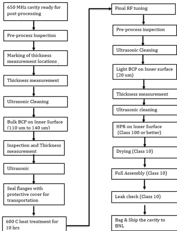
Figure 6: First post-processing procedure.
