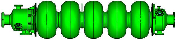
Figure 3: Engineering model of the cavity.
