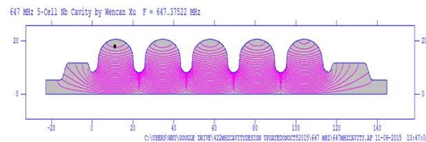
Figure 2: Superfish code model of BNL4 cavity.
