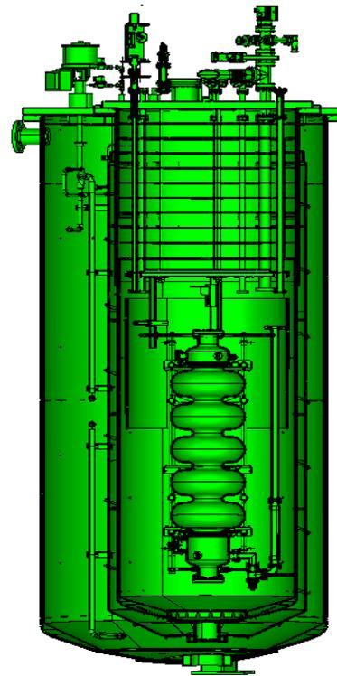
Figure 7: Vertical test dewar layout with a 5-cell 650 MHz cavity.
