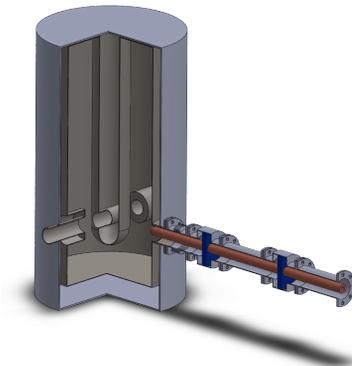
Figure 11: Assembly of the coupler.
