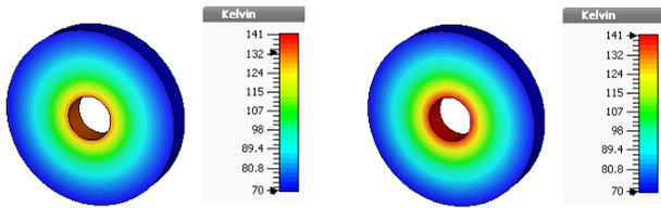
Figure 5: Thermal maps of the 70 K RF window without (left) and with (right) transmitting power.
