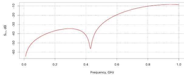
Figure 9: Full assembly reflection.
