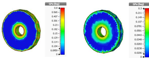
Figure 6: Mechanical maps of the RF window without (left) and with (right) transmitting power.
