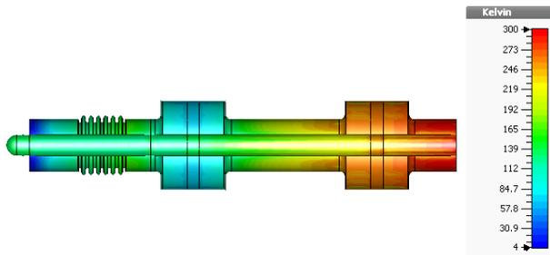
Figure 10: Temperature distribution in the coupler.
