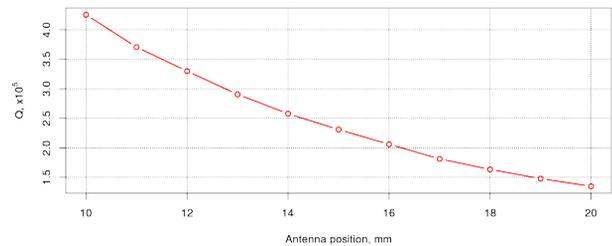
Figure 2: External Q-factor of the cell vs antenna position.
