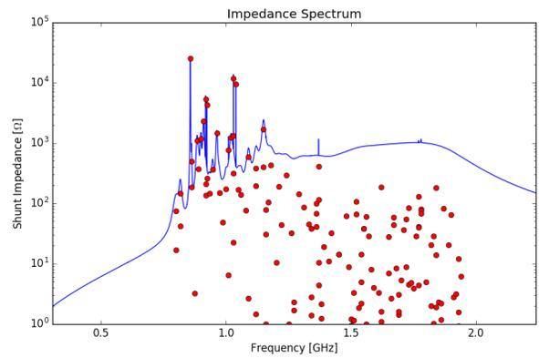
Figure 4: Eigenmode impedance results (red dots) and fitted impedance (blue line) for the Ring-Ring two-cell cavity with four beam line absorbers.
