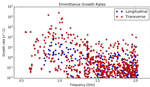
Figure 8: Beam instability growth rates are concerningly high due to the longitudinal and transverse impedance of the two-cell cavity.
