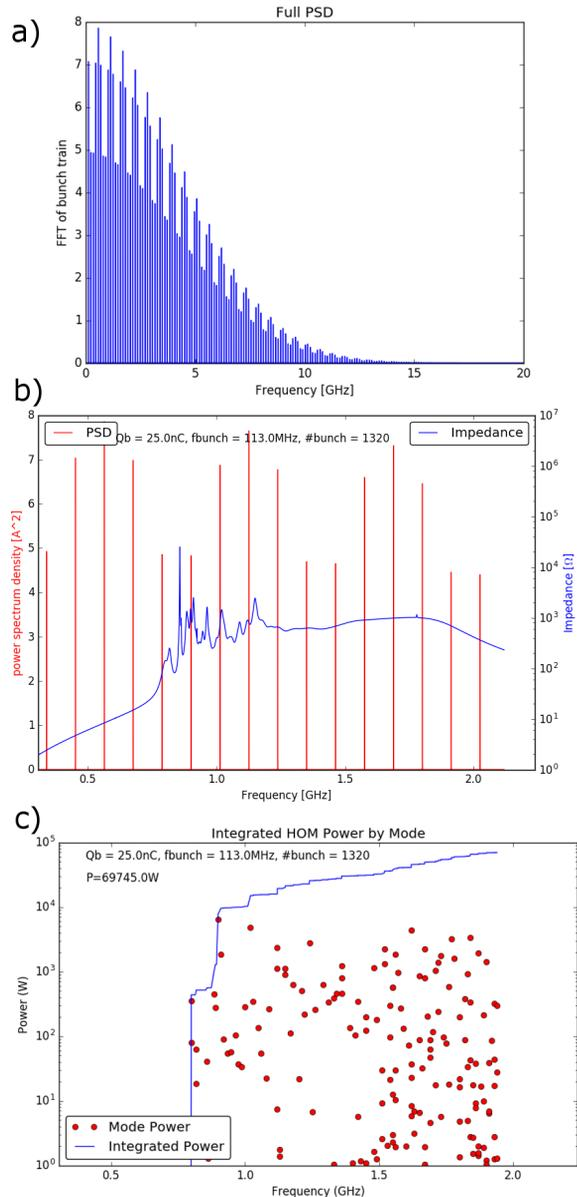
Figure 6: High luminosity scenario. a) full bunch power spectrum; b) bunch spectrum (red) overlaid with cavity impedance (blue); c) HOM power spectrum (red dots) and integrated HOM power (blue line).
