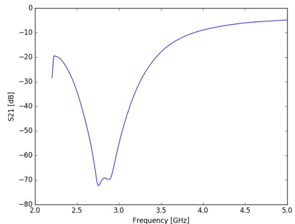
Figure 2: Transmission simulation for the LR beam line absorber with a resonance around 2.7 GHz to cover the peak in bunch spectrum power.
