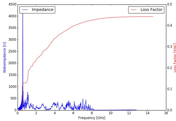
Figure 7: Wakefield impedance (blue) and integrated long. loss factor (red) calculated by CST and ABCI with a 50nC, 8mm long bunch. The loss factor is integrated to 0.44V/pC.
