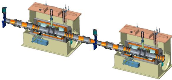
Figure 3: Conceptual drawings of the Ring-Ring eRHIC cryomodule assembly. The 2cell cavity is surrounded by a 500mm long warm-cold-transition with bellows (orange), followed by the first absorber, a section of beampipe, the second absorber and a downtaper section to a gatevalve.
