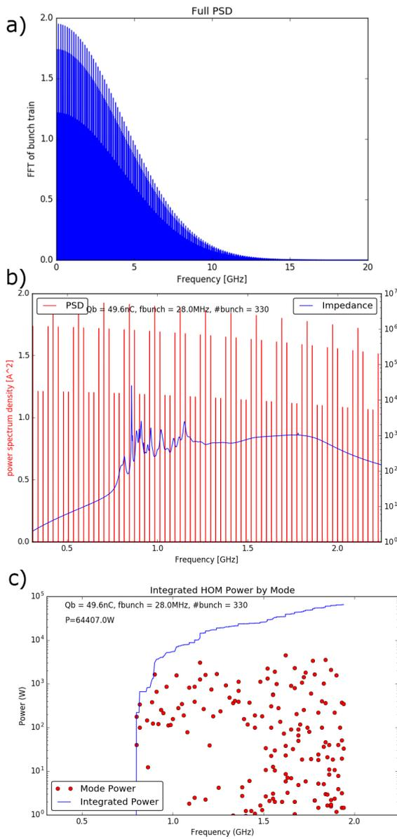
Figure 5: Medium luminosity scenario. a) full bunch power spectrum; b) bunch spectrum (red) overlaid with cavity impedance (blue); c) HOM power spectrum (red dots) and integrated HOM power (blue line).
