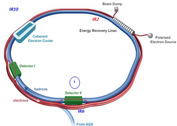
Figure 1: Layout for the Linac-Ring eRHIC with the existing "blue" hadron ring and the electron ring in red. The SRF Linac is located at IP2.
