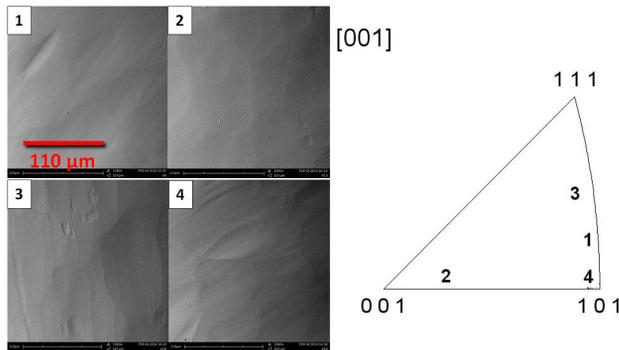
Figure 4: SEM images of four single crystal niobium samples received accumulated 90 minutes of BCP at 22°C. The orientation of the four single crystals is marked in the inverse pole figure.
