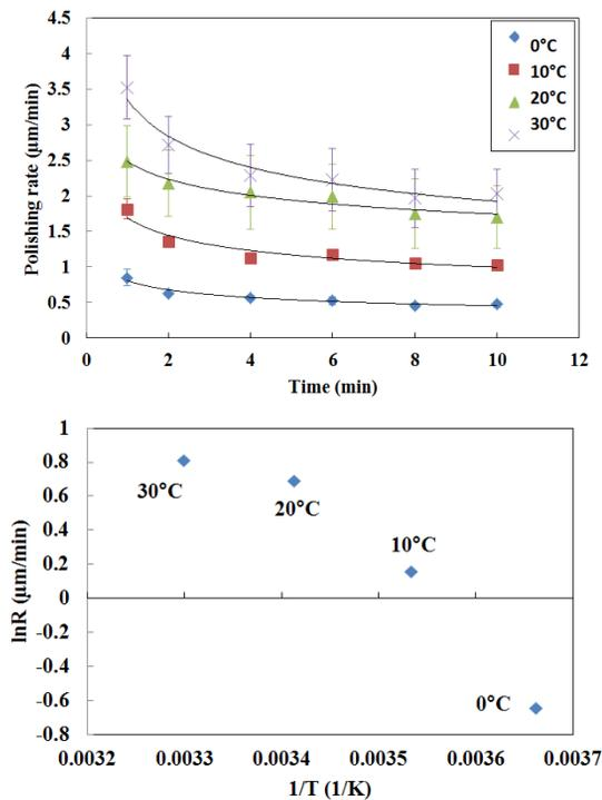
Figure 1: Nb BCP polishing rate as a function of time at 0-30°C. The natural logarithm of polishing rate as a function of inverse temperature (polishing rates at 6 minutes were used here).
