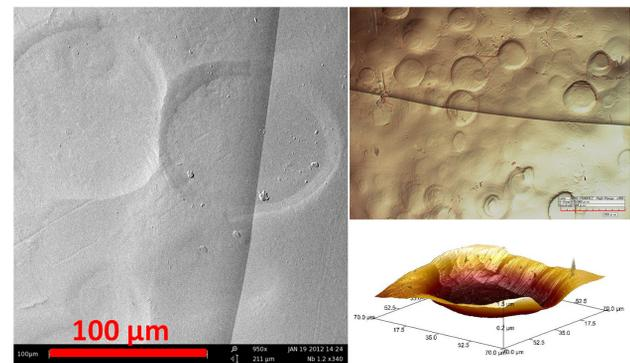
Figure 7: SEM, optical microscope, and AFM image of bubble prints on bi-crystal niobium received 80  $\mu\text{m}$  removal at room temperature.
