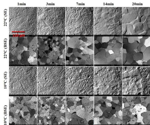
Figure 2: SEM images of fine grain niobium polished for 1-20 minutes, at 10°C and 22°C. For each sample, the upper image is from secondary electron and the lower image is from backscattered electron.
