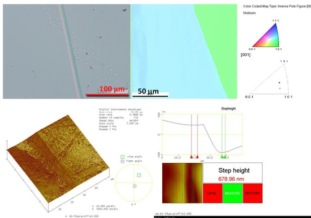
Figure 5: Optical image of a bi-crystal niobium sample after 12 minutes of BCP at 20°C. EBSD and AFM scan on the bi-crystal shows the orientation of the two grain is close to each other and the step at the grain boundary is about 0.68  $\mu\text{m}$ .
