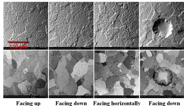
Figure 3: SEM images of fine grain niobium polished for 6 minutes at room temperature. For each sample, the upper image is from secondary electron and the lower image is from backscattered electron. The orientation of the sample was: facing up, facing down, facing horizontally, and facing down in the order of the images.
