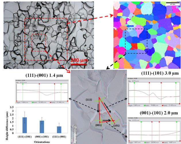
Figure 6: SEM image of fine grain niobium received 6 minutes of BCP at room temperature. EBSD corresponds to a 500  $\mu\text{m} \times 500 \mu\text{m}$  square area at the center of the SEM image. Height difference between the (111), (100), and (101) grains at the center was measured by optical microscope 3D profile function.
