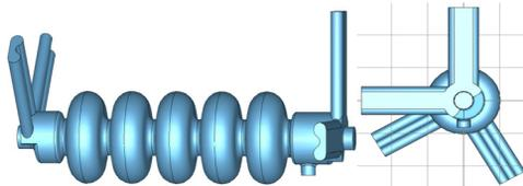
Figure 6: B-shape waveguide HOM damper.
