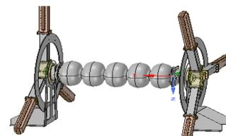
Figure 12: HOM damping measurement scheme.
