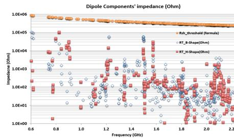
Figure 9: Impedance of Dipole components of B-shape and H-shape HOM damper.
