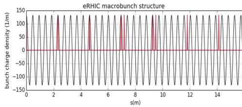
Figure 2: An example of the electron bunch pattern for the ERL-Ring eRHIC.
