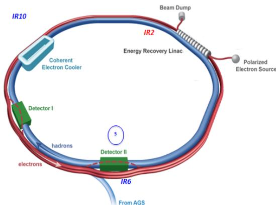
Figure 1: Layout eRHIC. Existing “Blue” hadron ring (center); Electron ring and SRF linac at IP2.
