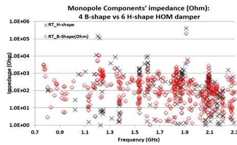
Figure 8: Impedance and HOM power comparison of the H-shape and B-shape HOM damper.
