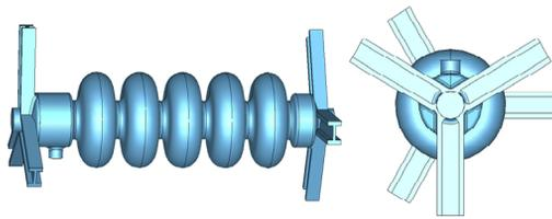
Figure 4: H-shape ridge waveguide HOM damping scheme.
