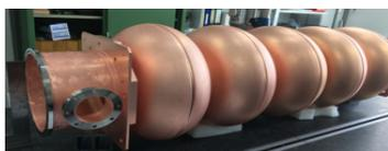
Figure 11: Copper cavity with detachable beampipe for HOM study.
