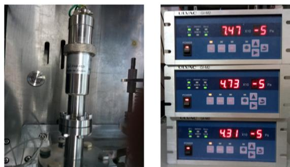
Figure 7: Vacuum gauge sensor (left) and ULVAC vacuum gauge (right).
