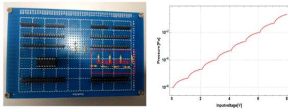
Figure 8: The front end of signals input (left) and detected voltage – vacuum curve (right).
