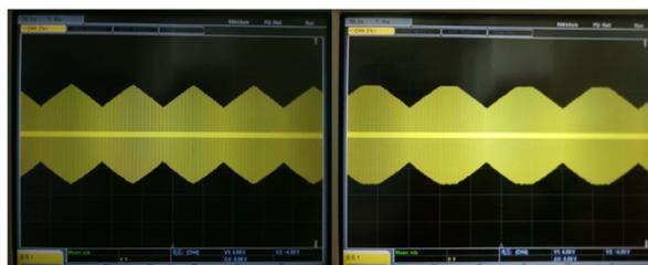
Figure 5: RF power signal picked up from directional couplers.
