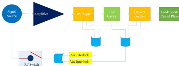
Figure 9: Overall interlock logic loop.
