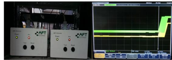
Figure 10: Arc detectors (left) and response-time test result (right).
