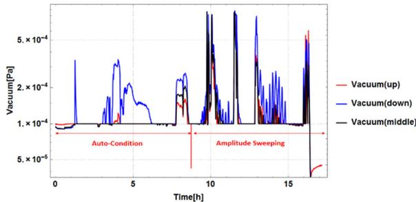
Figure 12: Vacuum variation of 16 hours of test result for LLRF control system.
