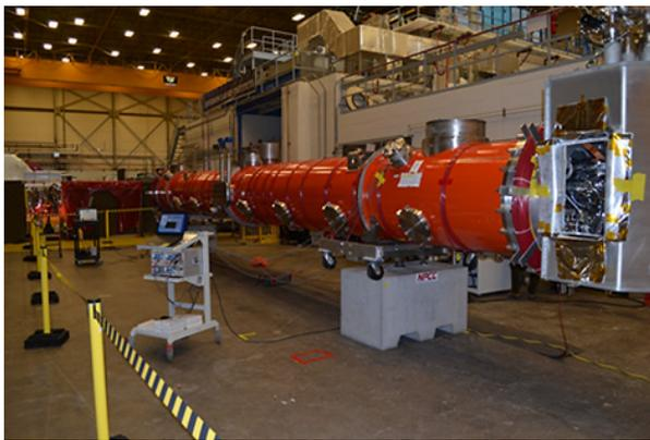
Figure 6: De-Gaussing of Prototype cryomodule. Cart in foreground is monitoring magnetometers in cryomodule during the process.
