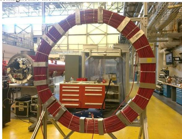
Figure 4: A mobile VV demagnetization 100-turn coil.
