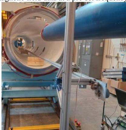
Figure 3: Motor-driven VV magnetic field mapping system.
