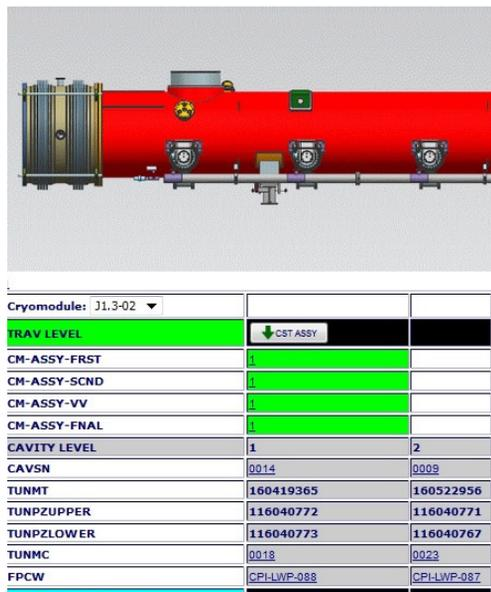
Figure 5: Cryomodule Drilldown and Summary Report.
