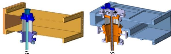
Figure 4: Original (left) and new (right) version of the SOLEIL cavity IPC.
