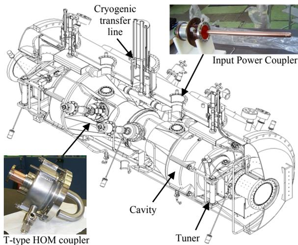
Figure 1: 3D-layout of the SOLEIL cryomodule.
