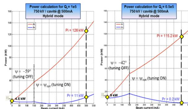
Figure 5: RF power versus  $I_{beam}$  with original IPC's (left) and upgraded ones (right) for  $V_{RF} = 3$  MV (750 kV/cav).
