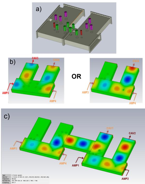
Figure 6: Magic Switch principle.
