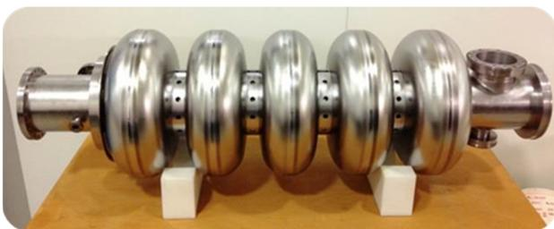
Figure 1: High beta 704.42 MHz undressed cavity.
