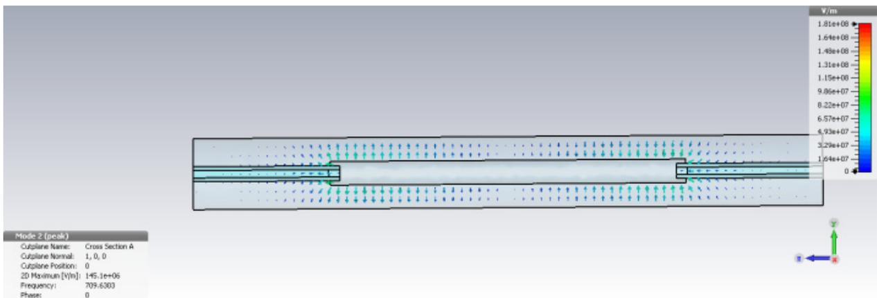
Figure 7: Cross section through the niobium coaxial resonator showing the Electric field pattern.
