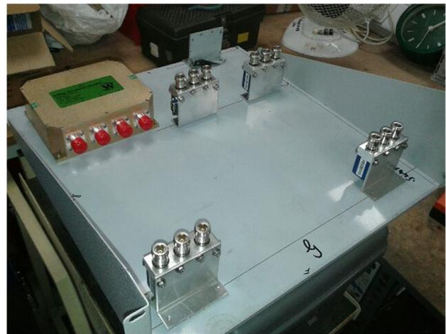
Figure 5: High power switching network in construction.
