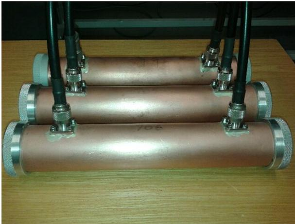
Figure 3: Copper coaxial resonators for validation.
