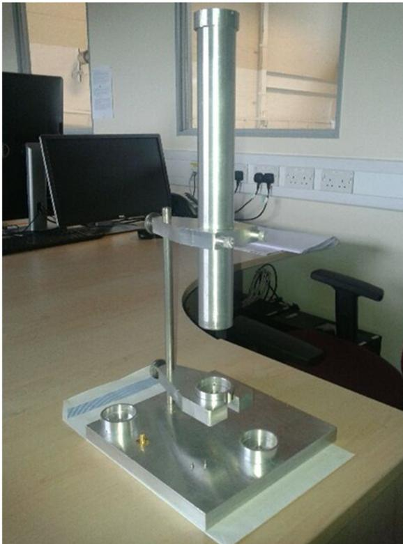
Figure 6: Dummy aluminium coaxial cavity.
