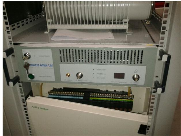
Figure 4: The 500W amplifier and load.
