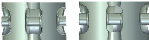
Figure 5: Rounding in the drift tube 5 mm (a), 20 mm (b).
