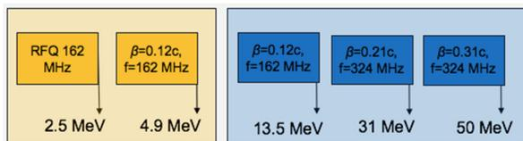
Figure 1: Proposed NICA injector layout of normal (left) and superconducting (right) structures.
