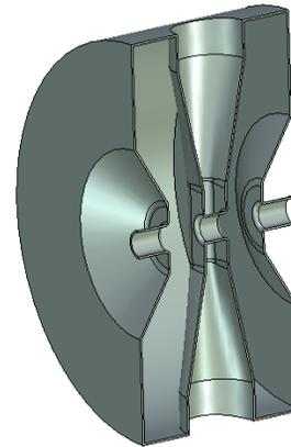
Figure 3: Spoke cavity for  $\beta=0.21$ .
