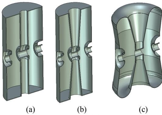
Figure 4: Three type of the HWR for  $\beta=0.21$ .
