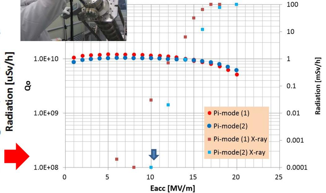
**By reassembly work, the onset decreased from 18MV/m to 10MV/m maybe due to our poor reassembly work**
