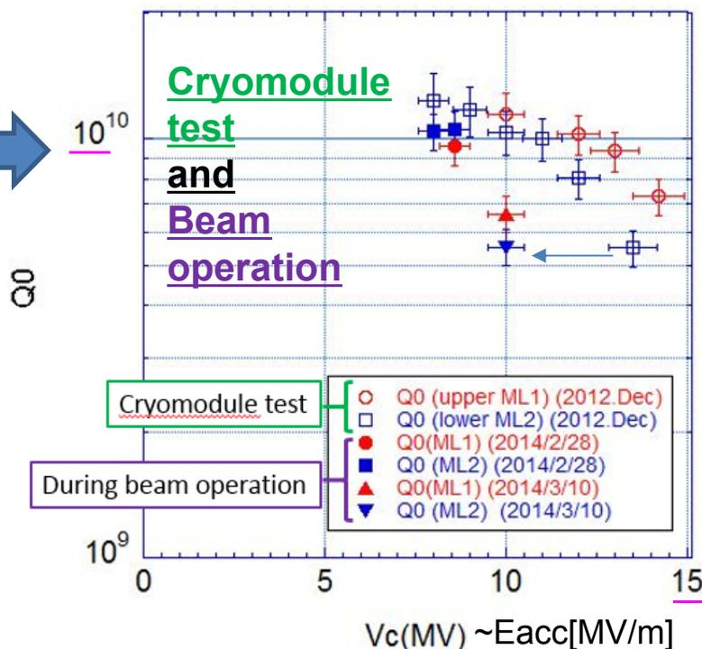
**Degradation** was observed **not only on string assembly** but also **beam operation**
