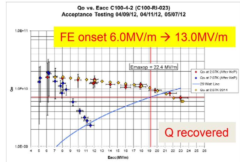
He process results on C100 cryomodule test @H.T M.Drury, TTC meeting 2014 March @ DESY
