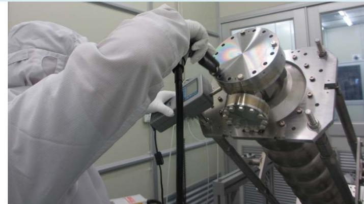
All screws of flanges of SS316L were plated by silver and ultrasonic cleaned and browed by ion gun to particles 0
