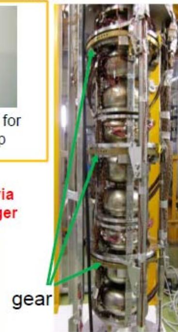
82 PIN diodes and 93 Carbon resistors are mounted on the mapping system along a meridian to detect 9cell radiation and temperature mapping precisely
