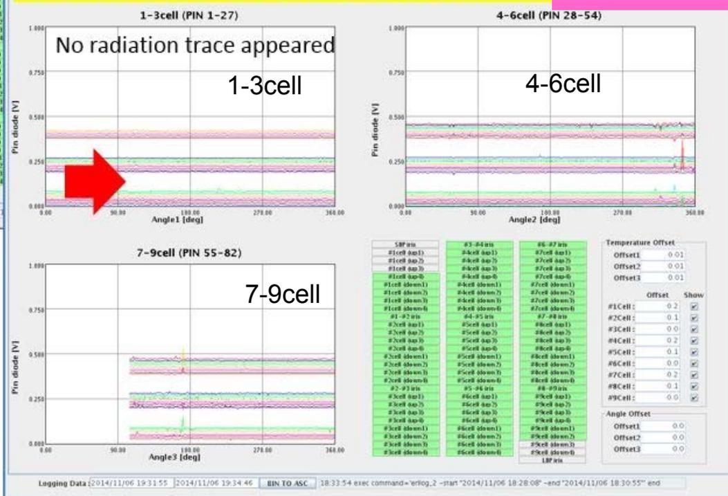
Finally every emitter disappear at 18 MV/m after RF process
