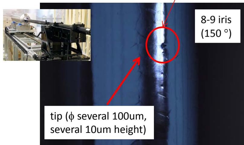
Tip was observed on opposite side of x-ray sharp peak by inspection.
