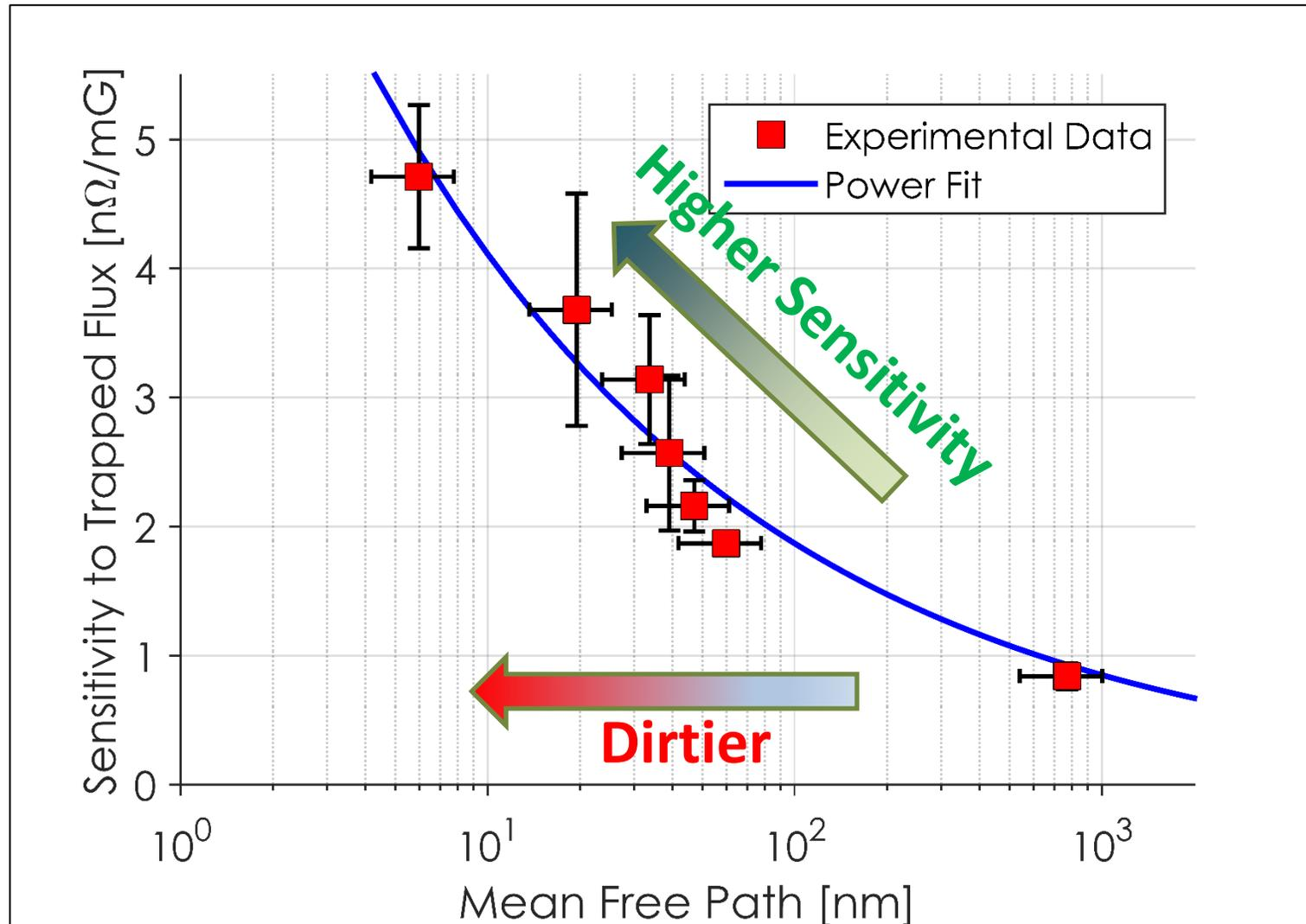
**Smaller mean free path results in higher sensitivity to trapped flux.**
