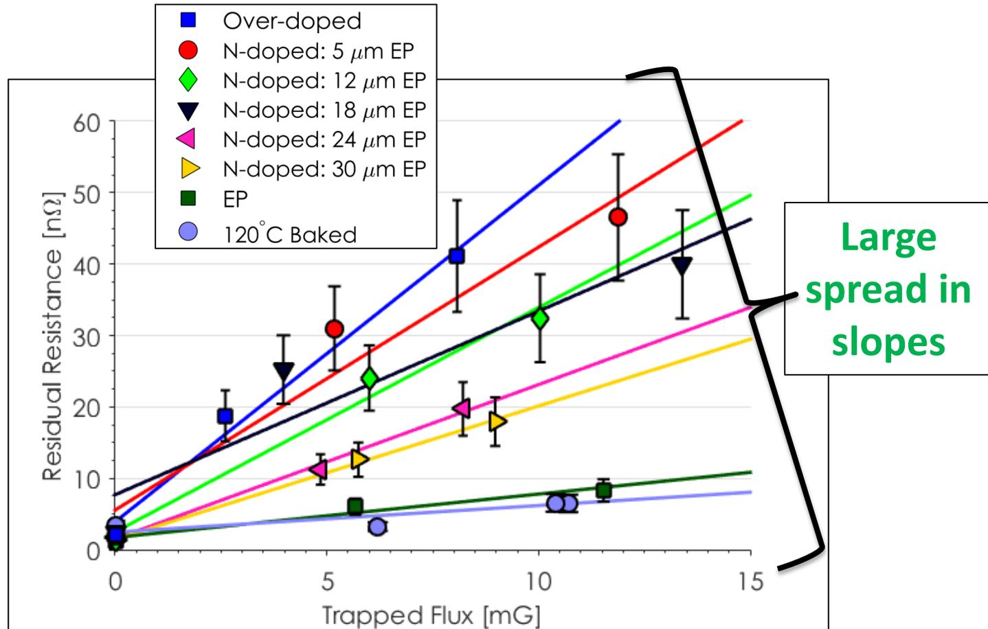
Cavities with different preparations show very different sensitivities to trapped flux!
