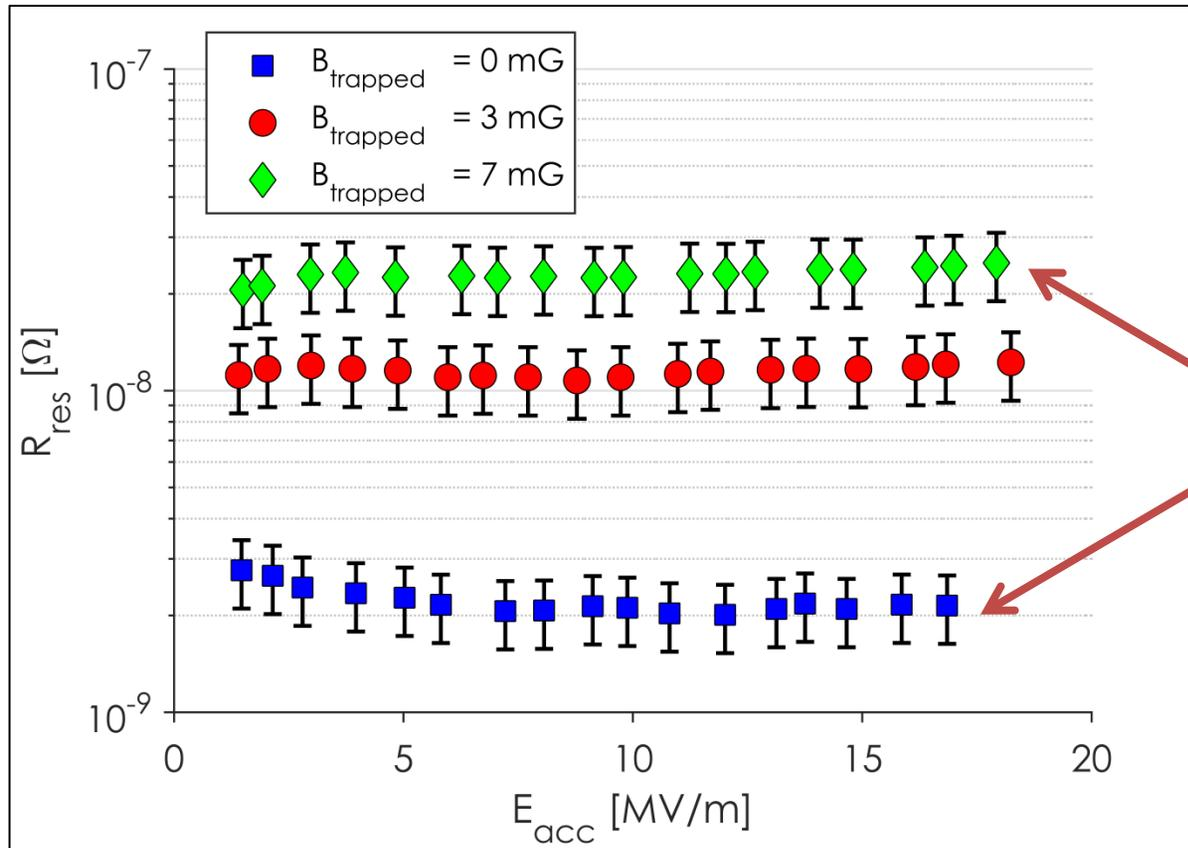
Residual resistance from trapped flux is independent of  $E_{\text{acc}}$  up to medium field
