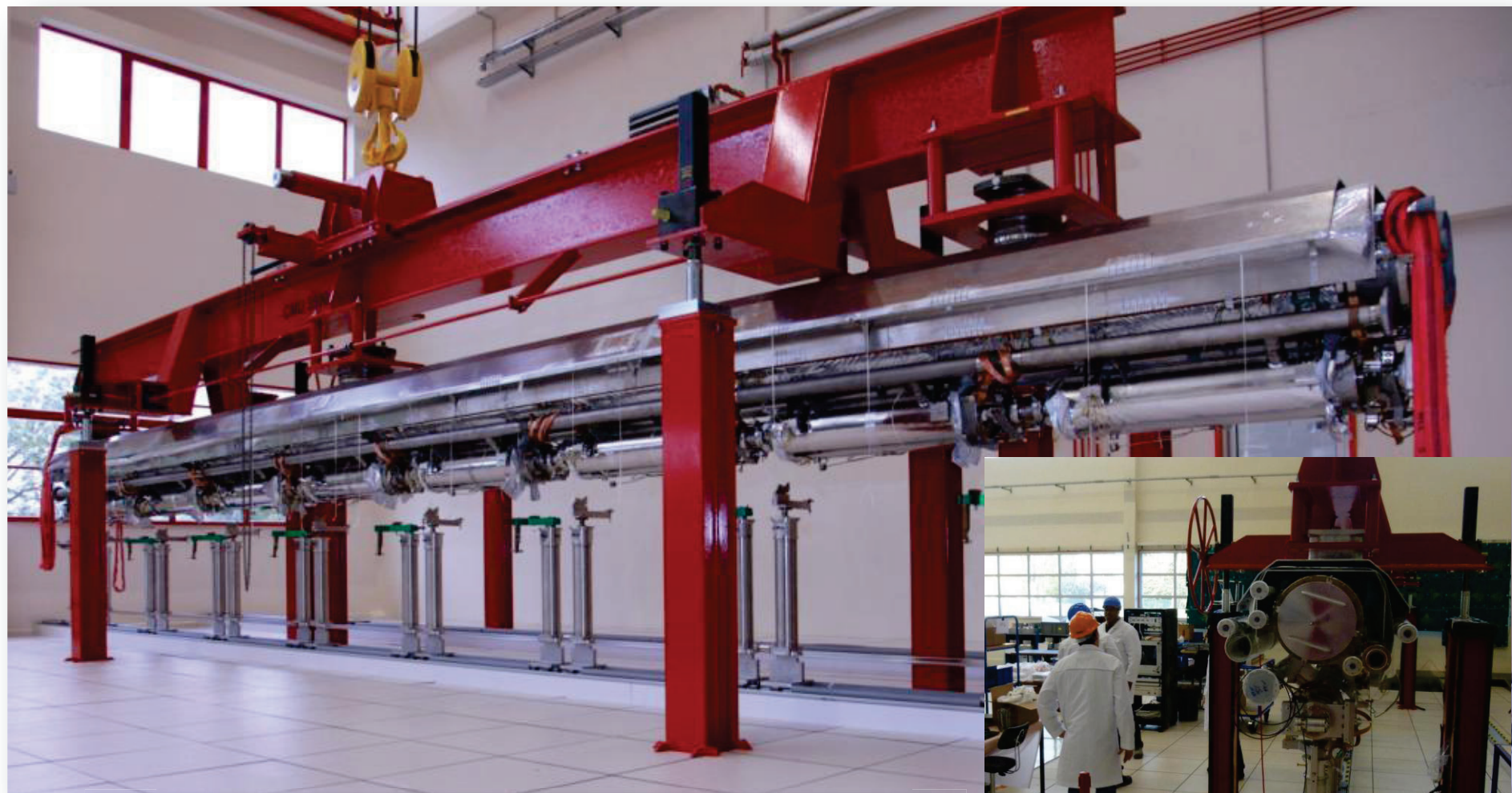
String roll-out and cold mass assembly (RO-WS)
