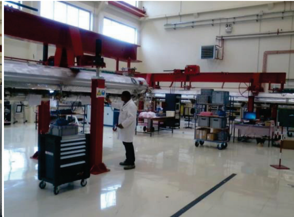
Roll-out (RO-WS) and Cavity alignment (AL-WS) workstations
