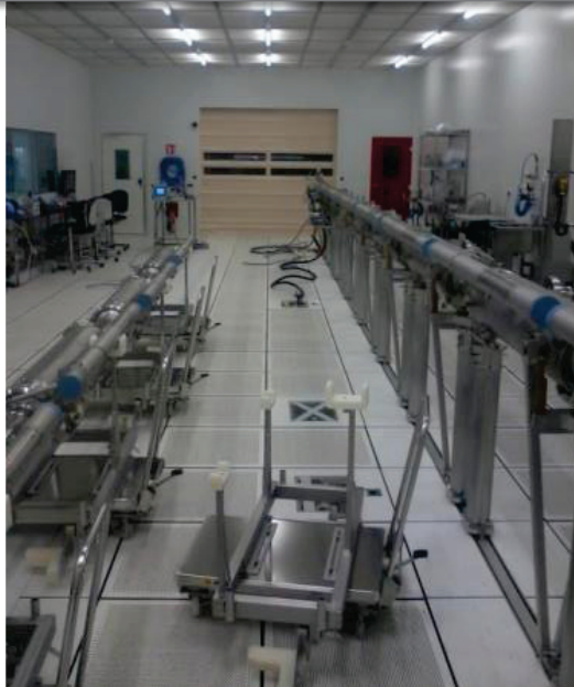
Cavity string assembly (SA-WS)
